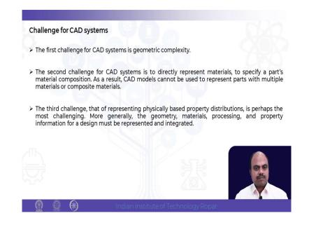
So, what are the limitations of CAD model, CAD systems? CAD system which is there (Refer Time: 30:09) ideas, Unigraphics, UX, NX, SOLIDWORKS, CATIA, Rhino. There are so many softwares which are available. However, many other software are not really designed to take care of the additive manufacturing process, because in a CAD CAD software many of you would have used it, that if you want to make really complicated shape, this is sometime is difficult using CAD, CAD model. It will take lot of time.
