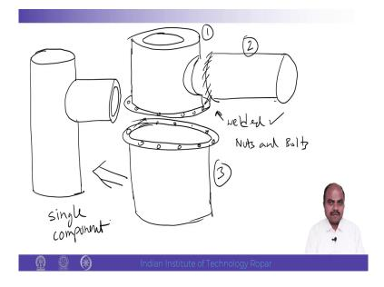
Imagine there is one component and it is having a hole here. So, down of it this is made using there is one another one similar to this. And, there is one another component is coming like this and this will be welded in this place. So, now instead of having this, this one what we can have? We can using additive manufacturing, we can have instead of all this one we can have single one.
