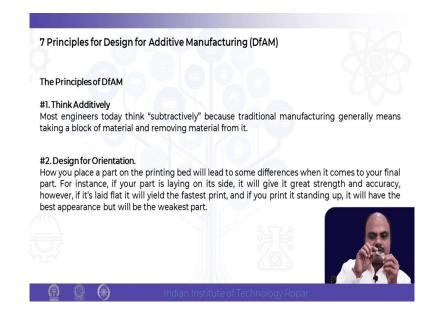
Now, 7 principles of additive manufacturing process. First is think additively. Previously, we should think subtractively which means that whenever a component is there, we used to think that how can I make this component. So, let us say I have this component, previously I should think that ok I have this rectangular bar and then I am going to use a method to cut.
