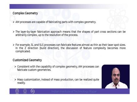
So, complex geometries we can make. So, layer by layered complex geometry we can make, but you should also understand that Z direction, the strength of the material in the additive manufacturing process is different in different directions depending upon the kind of component material machining process which we are following, that we should understand.
