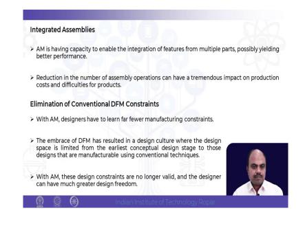
So, in integrated assemblies we can make where additive manufacturing process is actually enabling integration of features whereas, in traditional manufacturing process if you want to do it, you have to do it in different different components and assemble it. So, it is going to reduce the cost a lot.
