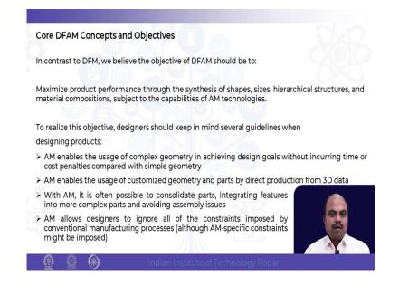
Now, in contrast to DFAM that is design for manufacturing, we design for manufacturing the normal design for manufacturing we are actually making a products. But, in design for additive manufacturing we are maximizing the product performance using synthesis of the shapes, sizes, hierarchical structure and then subject to capabilities of AM manufacturing process.
