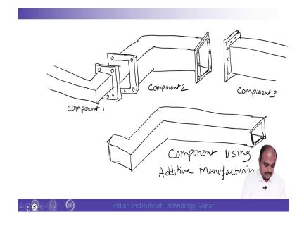
And take for example, that we are going to have this kind of component. Let us see this is water housing pipes and this is junctions. These are screwed with respect to each other. Here, third component is component 1, component 2 and this component 3. Now, instead of having so many components and having screws to join it, we can just use a single one and that is going to be like this something like this.
