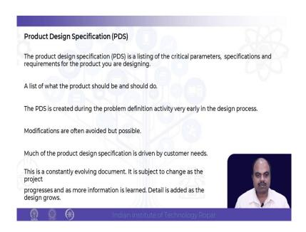
So, the product design specification is basically a document which is very important. After need identification, at the end of the need identification, we are going to have this document. So, this document is having a listing of critical parameters, specifications and requirement for
