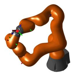
Although the end-effector achieved the desired position, the orientation is different in both the cases.
