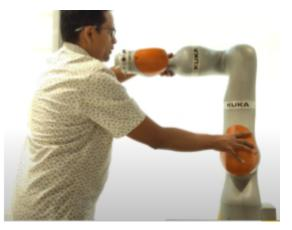
So, let me show you a small video here, which will clear it up very well, okay? That experiment that I have done, so this is the video. You see the whole of the robot is moving, but the end effector is stationary. There is no velocity at the end effector, okay?
