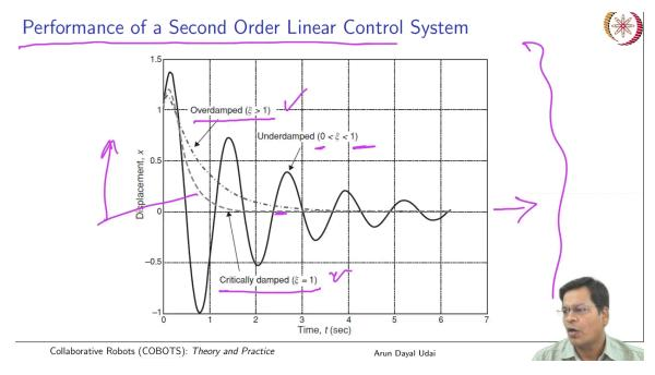
This is what the performance of your control system is. So, you can quickly write it as Displacement is plotted here, and your time varies like this. You see, you have an overdamped case for xi greater than 1, an underdamped case for xi lying between 0 to 1, and this is the case that was critically damped, where xi is equal to 1. So, in that case, it is a critical time, and in this case, the system settles to the desired value very quickly.
