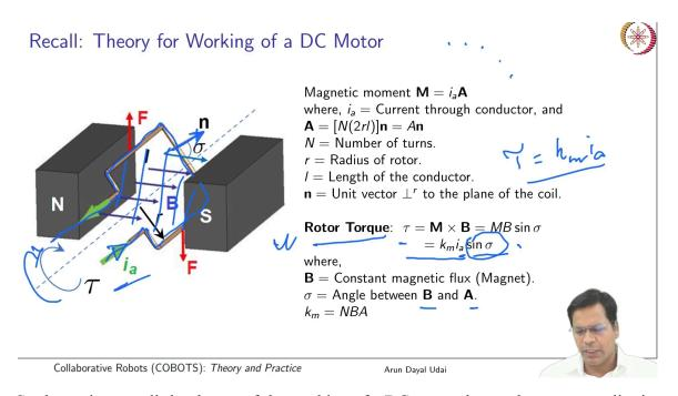
So, let us just recall the theory of the working of a DC motor that we have seen earlier in Module 2. So yes, this is the first thing that we have learned. So, we saw the structure of a DC motor. Basically, it contains a simple armature coil that is shown here, and you see it has a current that flows into there, given by  $i_a$ , which is the armature current. It comes out from here. It develops a torque, which is given by tau.
