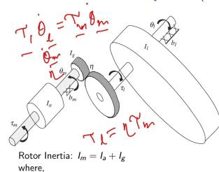
$I_a = Inertia$  of actuator and  $I_g = Inertia$  of gears
