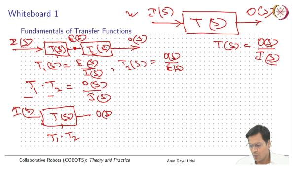
So, let us start. So, transfer function, you know. It is input that is I(S), and you have a transfer function, as you have seen. It is the Laplace of output by input. So, it is output Laplace. So, output by input, transfer function is given as.
