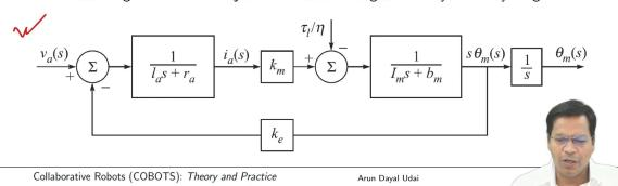
So, now let us get the transfer function of the joint so that I can get the input and output relation for this DC motor system. That is the whole of the actuator here.
