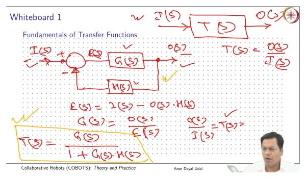
Now, let me draw it in a closed-loop way because the way we want to do it now is a closed-loop application. So, this becomes your input that comes here to the summing block over here that is plus. This goes to the Transfer function, which has G(S), and that is your output. You have a tapping from here that comes through a feedback line, which is here, that is, H(S), and that comes here with a negative sign. So, this is your input, and this is your output.
