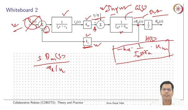
Again, look at it otherwise. This time, let us say it is driving by itself. That is, it is being driven by the load. So, in that case, you are not applying any external voltage. So, this is totally absent. So, in that case, the load torque will be visible. With the gear reduction ratio, it is coming onto the system. Mind it. So, this is always there. So, this is the driving torque, and the whole system is now getting driven by that.
