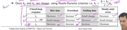
So, the Gain Selection for the PID controller that works is known as tuning of gains. So, you tune your gains now. So, the common design thumb rule is to set Ki as equal to 0. Start with no integral gain.
