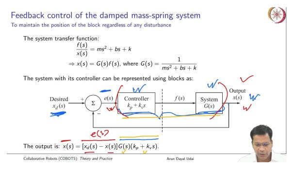
How was your system? Your system was very much like this. So, it was a force that got into your system. So, this is your system. Gain for, which is given by G(s), is equal to 1 by ms square plus bs plus k. You know that already. So, input was force to that. Output is the displacement that you can measure. So this is your system. You already have a controller that is given like this. So, can we put everything in place now and represent the system as this? You see what it is now.
