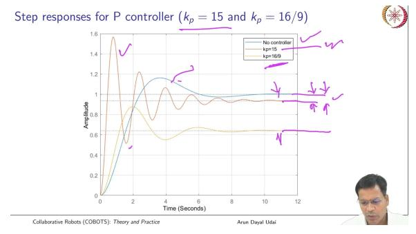
So, I can see the plot, which is very much like this. So, with no controller, this is the system, okay? The blue one, and with Kp equal to 15, it is the red one. So, you see, Kp is higher in this case. Kp is very high. It is 15.
