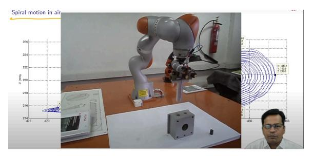
Let me just show you how it behaves in the air. So, it does a mark here. I will not establish any contact. I will just go on top of the surface, and this is why I have not lowered. That means I have not put the vertical motion, and it is a diverging and converging spiral. This is the visible displacement. So, this is a force spiral. If you hold it, it tends to stop because of external forces that you are applying at the end effector. So, this is a spiral search path.
