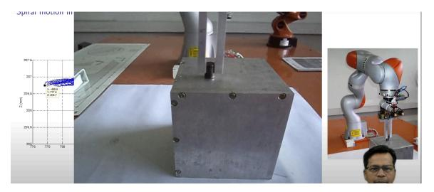
So, this time on the surface, you see again it will lower with a certain velocity, establish contact, maintain a constant reaction force, and it is doing the spiral diverging and converging search.
