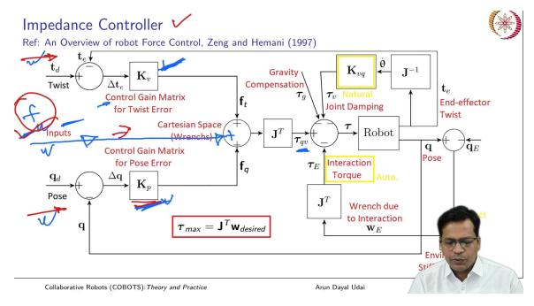
So, let me come back to the impedance controller here. So, this is my impedance controller. So, you have seen the effect of pose error that which is exactly the stiffness controller, which is here, and apart from that, you have impedance, which is here. You can have both. So, combined, it makes things stable, makes everything stable. So, it has no more tendency to bounce and create any jitter while it is contacting.
