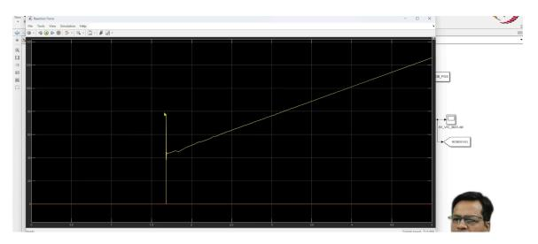
So, immediately upon contact, a huge amount of surge is there due to collusion and then the force rises gradually with the wall because the velocity is increasing as it approaches the robot, and it compresses the robot. So, the higher the velocity higher the force it generates. So, this is what is expected out of impedance.
