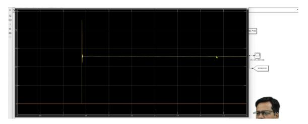
So, let me check the plot here. So, you see it is a straight line because the velocity is constant, and I have not set any stiffness along the interaction direction. I have not set any stiffness anywhere. So, only because of damping because which is proportional to the velocity. Velocity is constant; force has to be constant. So, this is generating a constant force interaction force and the robot is continuously moving along with the wall.
