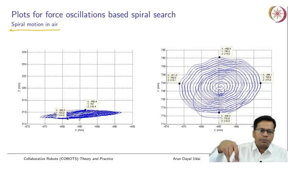
So, let us observe closely how the motion could be when it is in the air. In the air, there is no resistance. So, it tends to create a spiral path of some size.
