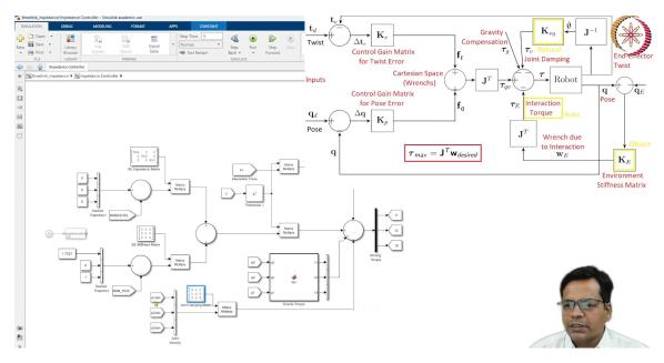
So, let us get into the impedance controller directly. I'll just open up the picture here so that you can refer to it quickly. So, here is the trajectory the desired trajectory input. This
