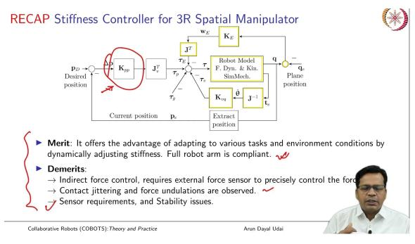
Just have a quick recap on the stiffness controller for the 3R Spatial Manipulator that we did. So, you see, it has a few merits. It offers the advantage of adapting to various tasks and environmental conditions by dynamically adjusting the stiffness. You can dynamically adjust this (Kpp) because it is all implemented in software. So, you can
