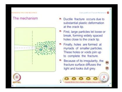
Now, let us look at the animation, explaining the phenomenon of ductile fracture. We have seen already that ductile fracture occurs due to substantial plastic deformation at the crack tip, and what you have is, first the large particles, let loose or break, forming widely spaced holes close to the crack tip. In fact, you could look at the animation simultaneously, but you would also spend time and looking at the animation exclusively later.
