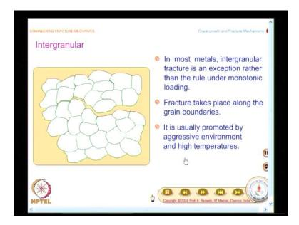
So you will have to understand under monotonic loading, it is only an exception. And in the case of intergranular, fracture takes place along the grain boundaries. And this is, usually promoted by aggressive environment and high temperatures. We have already seen in some of these, in the context of crack growth. In the case of fracture also, aggressive environment and high temperatures induces intergranular type of fracture.
