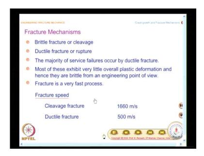
Now, we move on to fracture mechanisms. We have already noticed, that there are 2 important fracture mechanisms; one is brittle fracture; another is ductile fracture. Brittle fracture is known as cleavage, ductile fracture is also known as rupture. And we will see,
