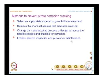
So, the first step is, select an appropriate material to go with the environment; and the second step is, remove the chemical species that promotes cracking. These are all doable. And the third step is, we have already seen, in the case of active path dissolution; tensile stresses causes the correct environment for the crack to grow.
