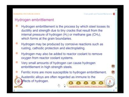
The next process is Hydrogen embrittlement. This is another possibility, by which the cracks can grow due to stress corrosion cracking, and what you find is, hydrogen embrittlement is the process by which steel looses its ductility and strength. What happens? Tiny cracks that result from the internal pressure of hydrogen or methane gas causes loss in ductility and strength, and where do these form? Again, the grain boundaries are affected.
