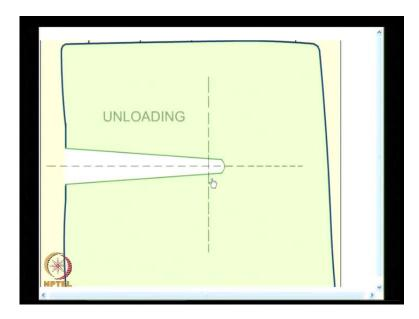
So, you have, while the crack is loaded, it gets blunt; during unloading, it gets sharper. So, this opening and closing leaves the mark on the material, which appear as striations.
