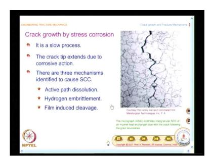
Let us continue our discussion on stress corrosion cracking, and we have looked at, in the last class, crack grows by a stress corrosion, and we saw that, it was an inter-granular
