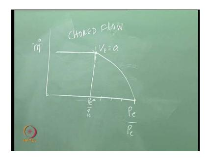
Let do this experiment, let say I now plot the mass flow rate through the nozzle, that means, the rate at which mass is getting sucked out as a function of let us say the value of P e that is the exit pressure to the chamber pressure.
