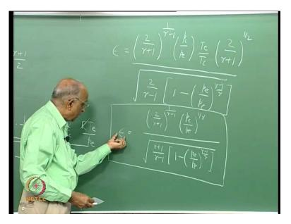
And therefore, I can write this as equal to P c by P e to the power one over gamma and therefore, my net expression now becomes 2 over gamma plus 1 to the power 1 over gamma minus 1 P c by P e to the power 1 over gamma divided by gamma plus 1 divided by gamma minus 1 into 1 minus P e by P c gamma minus 1.
