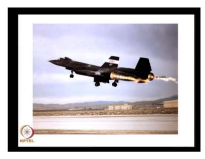
I just continue with this, it shows SR-71 which is the plane. I see the shock diamonds over here, in this particular case. And we continue with this, this is a test of an engine. And here you find, there is a shock here and something like this. This is because the exit condition is either under expanded or over expanded.
