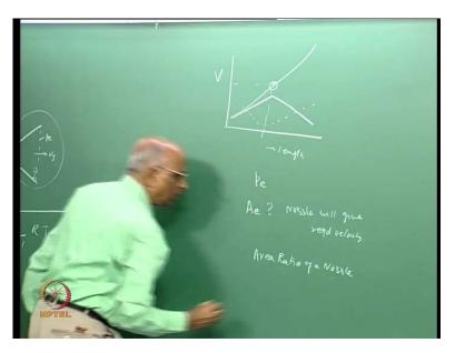
The velocity of the gases as a function of the length of the nozzle mind you along the length of the nozzle initially I have a converging shape then I have a throat then I have the diverging shape this is I get the sonic velocity and therefore, the velocity will keep increasing along the nozzle.
