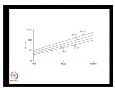
I put it for larger value of pressure ratio here again the value is P c by P e as a function of the area ratio, you find that as gamma decreases I need a larger value of the area ratio. In other words what it tells me is if my gasses have a smaller value of gamma then I need a larger area ratio to give me the same value of pressure ratio. I think this is all about area ratio.
