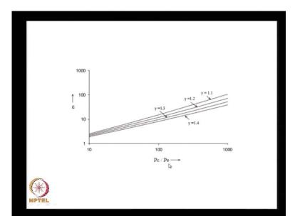
I get the area ratio as a function of P c by P e as P c by P e increases the area ratio increases and in fact as the gamma decreases from gamma of 1.4 to 1.1, I find a larger area ratio is required to give me the same value of P c by P e.
