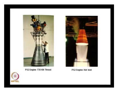
See this shows a particular second stage of PSLV, and here you see this is the divergence portion of the nozzle, which is chronicle nozzle. This is the compression chamber. And if I take the inside configuration of the nozzle, it will have a throat and will come back like this to the chamber. Therefore, I am looking at the outer portion of the nozzle here.
