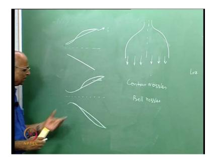
this divergence angle over here and in the initial stages what I do is, I expand it like this and bring it back like this; that means, I expand it out and bring it like this or the shape looks something like a bell; the shape of the nozzle looks like a bell here; I am sorry the figure is not. All right, this is the center line; how does a bell look like? Like this. Initially, I expand it out; I decrease the divergence angle such that the flow goes out actually.
