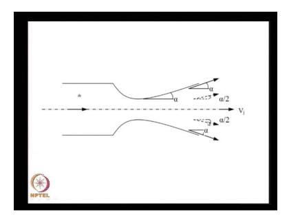
I will not get into detail but, I will just summarize it through series of, may be slides over here. In the first slide here, I will show the divergence losses, may be, alpha and how we got the divergence losses coefficient. This was the value of delta, which we decided as percentage loss in thrust versus the angle alpha.
