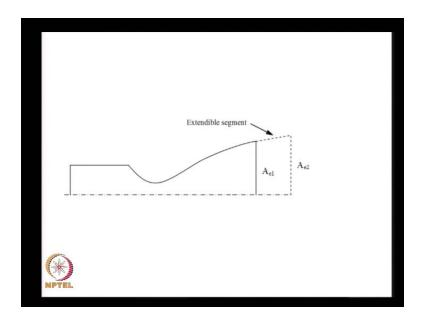
Initially, I have a small area ratio corresponding to A e1. I store this on top of this and when I want to fly at higher altitude, I push it out and I get a larger value of this over here.
