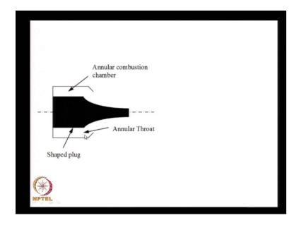
This is what we say is a plug nozzle or a spike nozzle. I have a spike over here. The flow comes. The flow in these cases, you know, you generate it in an annular chamber instead of having a chamber over here. I push the flow onto these inner surface and inner surface guides the flow. Outer surface is free; therefore, I can have any type of expansion what I want.
