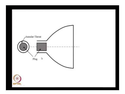
Those who are interested should go through it. This is a plug nozzle. I put a plug here and I have an outer surface, which guides the flow. The inner surface is free therefore, it can adapt to the flow where it where. What you have is an annular throat, instead of having a diametrical throat over here.
