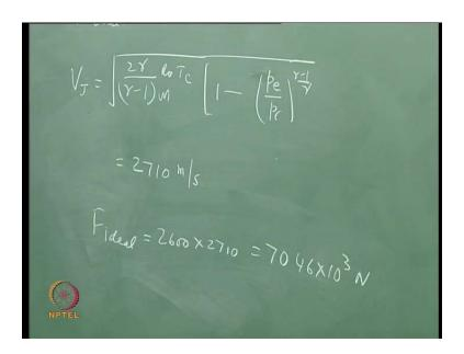
p e is equal to 0.1 m p a, p c is equal to the value what is given here that is 6.65 m p a. You substitute it and you get the v J is equal to 2710 meter per second. Therefore, what is the value of thrust? Thrust is equal to m dot 2600 kilogram per second multiplied by this. Therefore, the value of F ideal is equal to, multiply it m dot v J, which gives you the 2600, and let us write it down, into 2710, which is equal to 7046 into 10 to the power of 3 Newton.
