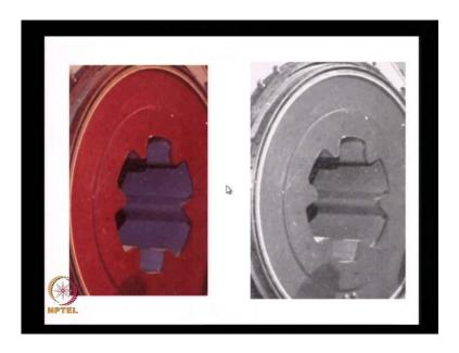
I could have grains, it could be of different shapes; maybe I could have lobe like this instead of having a star over here, I could have a lobe like this and what for what will happen in this case? The burning surface area, this is the inner surface of the grain, this is the length of the grain in this direction, the evolution of surface area would keep on evolving like this, keep on evolving like this until it touches the outer surface of the grain.
