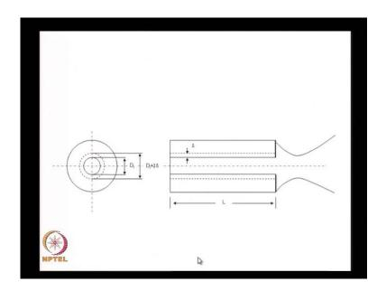
And, thereafter, we also evaluated how we could determine the pressure at different instance of time for the radial inward burning grain and also the time taken to consume the propellant from the inner diameter D i to the outer diameter D o.
