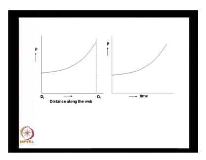
Having said that it is not possible for us to determine the pressure variation along the grain, let us go back. You know the distance between the inner surface and the outer surface is what we call as the thickness of the grain and the minimum thickness is what is known as a web thickness; I will take a look at it again today. And, if I say this is the
