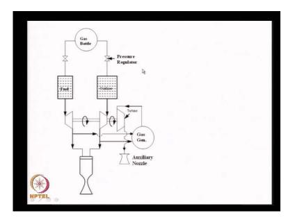
And therefore, what we do is we take the fuel, we take the oxidizer, we pump it into it. I remove some fuel from the fuel line, I remove some oxidizer from the line, I burn these gases separately over here, generate hot gases. Supply these hot gases into your turbine,
