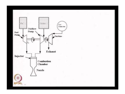
And therefore, what we normally do is, we need something like a gas generator which can supply work to a turbine and using the turbine I drive the time and therefore, it becomes a pump and a turbine and it is known as a turbo pump. I require another gas source, but to have a dedicated gas source is going to be a problem.
