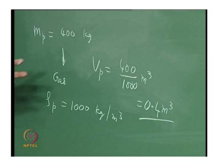
Let us calculate V P over here for this particular problem, V p if I take the density of the propellant to be same as water, density is equal to 1000 k g per meter cube that is the density of water 1 gram per c c. And therefore, the volume V P over here is going to be 400 divided by 1000 meter cube which is equal to 0.4 meter cube. In other words, for this rocket may be I have to get rid of 0.4 meter cube at a given value of pressure.
