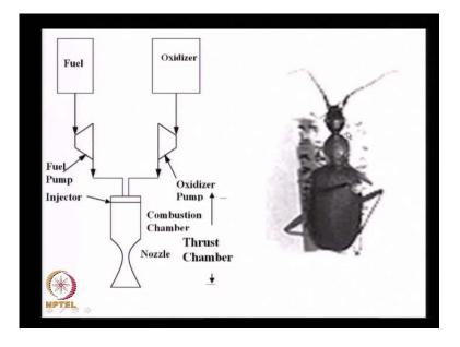
And if you look at what this beetle does, may be a chamber containing oxidizer, a chamber containing fuel, a third chamber in which it reacts and forms hot gases and squirts it out. Well, a liquid propellant rocket consists just a fuel in a tank, an oxidizer in a tank; you pump the fuel and the oxidizer into a chamber. And how do you pump it?
