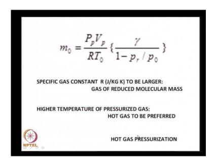
And said m o u mass of the gas required is equal to P p V p by R T 0 gamma by 1 minus p r by P 0 and then we found out that hot gas pressurization is an option.
