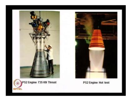
Well, this is all about it. Let us I thought maybe we should at this point in time itself look at few more pictures of this. Well, this is the engine which I just now showed you a liquid propellant rocket engine which is may be much taller than this man over here, this is the combustion chamber, this is the pump, this is the nozzle and this shows the rocket firing.
