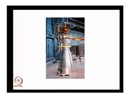
Well, this is all about things which I wanted to show, I show the U D M H N 2 O 4 rocket here. This is the chamber, this is the nozzle and these are the pumps supported.
