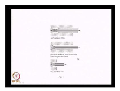
See these things are essentially when I have an orifice I have veen contracta here, flow attaching here. Sometimes even for the same length the flow go straight it does not attach whereas, for a small length is understandable, because if I cut the orifice here, well there is no way of attaching this is understandable, but this also takes place what is the reason for this let let us put it down.
