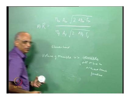
Let us say R mixer ratio is equal to the number of oxidizer orifices, into the area of each oxidizer orifice, into 2 into delta p across the oxidizer orifice, into the density of the oxidizer orifice divided by number of fuel orifices, area of the each fuel orifice into 2 of delta p across the fuel orifice into rho of this. If I have a shower head which has common delta p f is equal to delta p oxidizer and of course, 2 cancels and this is how you get a mixer ratio.
