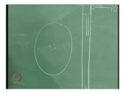
I have to put something like a sieve or something over here, such that may be the holes which are over here, are covered with a sieve such that there is more pressure drop and there is less pressure drop on the outside such that all the holes can have equal flow. And these are some common things which we use in the design of shower head injector.
