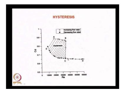
And if I do an experiment I start at low value of Reynolds number wherein I get an attached flow for which, since it is the attached the whole flow area is contributing to the flow and therefore, I get a high value of discharge coefficient it comes here. Somewhere cavitation starts it begins to separate I go over here it is still separated. And now when I start reducing the pressure or reducing the velocity again it goes like this, but it the
