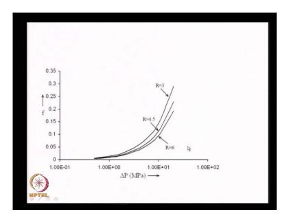
And we said as f the fraction of the propellant which flows through the gas generator as a function of p for maybe. I am considering the the delta p as point 1 MPa, 1 MPa, 10 MPa, 100 MPa it tends to increase. You know it is it is a linear with respect to delta p, but since I use a logarithmic scale the the values begin to show up as R increases the
