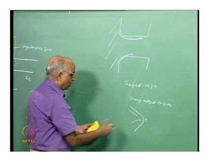
Let say an orifice like this this is the manifold. Why not make the orifice which is smooth streamline streamline along the flow, this will give you full flow, but to fabricate such things is difficult. I could have an orifice which is like this the next one would be different to get reproducibility in something like a shaped orifice is more difficult. And
