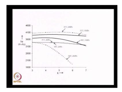
All what I am saying is. If I operate a gas generator cycle at a small value of pressure, this is the net value of specific impulse I get. If I operate the same engine on a stage combustion cycle at low pressure, I get a slightly better performance, because I have I have not lost very much, because f is still small. I have lost something from stage combustion cycle to gas generator cycle, I have I still find gas generator cycle is lower than stage combustion cycle, but the loss is small.
