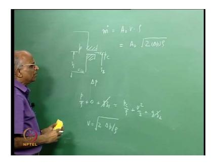
Which you all would have done in your fluid mechanics class, but let let us just try to do it. We have a manifold now I am considering the case of a single orifice, and I can just multiply it by n and get is my single orifice, this is my pressure here, this is my chamber pressure here. The difference is equal to delta p now I want to write an equation I say that the velocity here is 0, I form to find out the velocity here at the exit. I denote it by v I use
