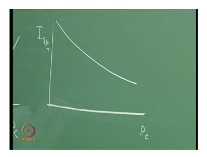
And we found g g was small if I increase this f the I T will decrease or rather I can tell myself in the gas generator cycle, if I by to plot the total specific impulse of your system as a function of let us say your value of p c. In your gas generator cycle even though the specific impulse will increase with chamber pressure.
