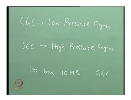
And generally for cryo engines may be 100 100 MPa or I am sorry 100 bar or 10 MPa seems to be the limit for a gas generator cycle, above this to operate a gas generator cycle you will lose more then what you can gain and this is how we do a cycle analysis.
