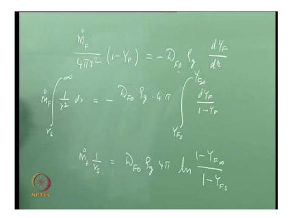
I now get the value of m dot of the fuel which is leaving into 4 pi r square, no divide it by 4 pi r square into 1 minus Y F is equal to minus diffusion coefficient of the fuel in oxygen multiplied by the density of the gases into dY F by dr, I play with this equation a little bit I simplify it and now I say dY F by dr is equal to minus if you please be careful.
