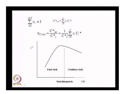
And give a value of eta C star due to distribution is equal to the net volume, as a function of the summation of the product of concentration and the C i value.
