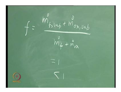
Therefore, now I say out of the total propellant which is m dot F plus m dot o, the thing which gets converted to vapor is equal to m dot of fuel which vaporizes plus m dot of the oxidizer let us say oxidizer which vaporizes, therefore the fraction of the propellant which really contributes to combustion is m dot fuel which is vaporized, plus m dot of the oxidizer which is vaporized divided by the total liquid which gets injected over here,
