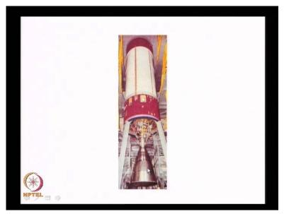
This is the large tank ages what is shown here, this is the pump, this is nozzle.
