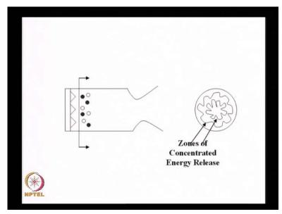
If I have a liquid propellant rocket, well I have injector; I have zoon of heat release like this. Therefore, I could have tangential and radial modes also causing this, and you could end up having pressure perturbations.
