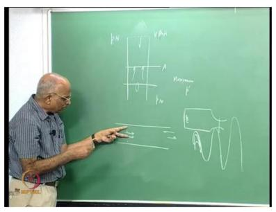
We found, that the tube in the vertical condition, may lot of noise. Where as in the tube which was in the horizontal direction also make some noise, but was not as I in the vertical tube what did we do. We put some heat source at some location, when I put some heat source, hot gases are converted of, hot gases are converted of, they meet this boundary, when I have the velocity node, it gets reflected. I get something like a pressure
