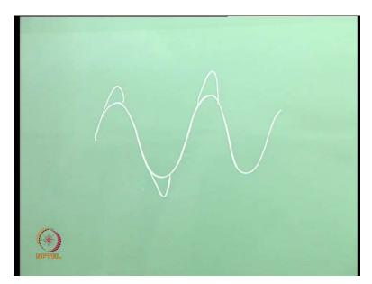
I could have velocity like this, what should I do if I have to increase the magnitude of velocity perturbation. Velocity perturbation is v prime, therefore if momentum, if rate of change of momentum; that means at this point I put more momentum into it, well could increase, here I remove, here I add; that means if the rate of change of momentum, could be put in phase with velocity perturbations, then my velocity perturbation could also increased.
