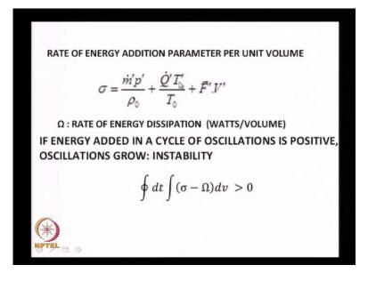
And we put the all these things together, we had a dissipation term and energy supplying term, over cycle of oscillations, if it is greater than zero, well and oscillation could occur. Only thing which is important for us to remember is, Q prime and p prime should have the same frequency, otherwise it is just not possible to have this.
