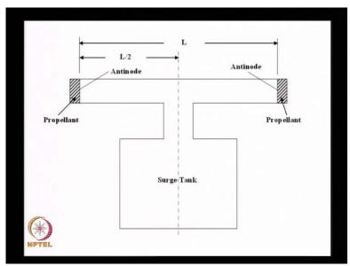
Inner to be able to figure out, how much of heat release, gets into the oscillations, we have specific devices. Now this is something which we must know, supposing I want to measure the growth constant of propellant, supposing I have let us say solid propellant in a chamber.
