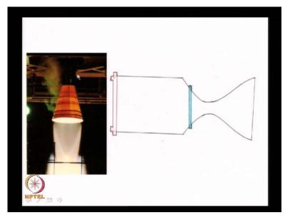
This figure shows, opening here; that means I slightly changed the tangential mode, because the dimension being inside here, and I put a slot. The dimension increases and this is been effective in reducing in the combustion instability of one of the Viking engines of 60 ton liquid propellant rocket. Let us go further, now we said there are different types of instabilities.
