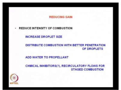
And let us now talk in terms of third type of instability, in which we said, instead of the wave mode or the bulk mode of instability, combustion instability could also be caused by process.
