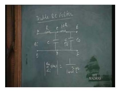
Here now the double RC filter we adopt when we are not getting the desired passage of the low frequency signal.
