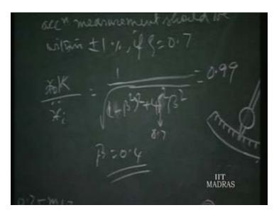
Now this is equal to 1% error so the magnitude ratio will be 0.99. So now substitute, size given as 0.7 and beta can be found out from this equation, except beta all the other are known so beta comes about beta is equal to 0.4, it's a straight forward problem. So with this we close the chapter on acceleration measurement.
