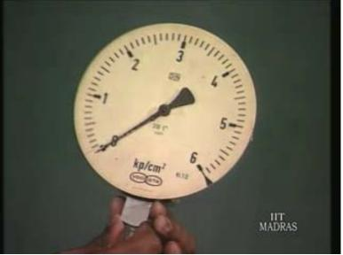
A typical example is what you have seen earlier a pressure gauge. It's a pressure gauge kilo point; it is kilogram force per centimeters. This is a 1 bar, 2 bar, 3 bar, 4 bar, 5 bar, 6 bar its range is 6 bar. It's an instrument pressure gauge typical instrument and if you open the back side you see all these elements.
