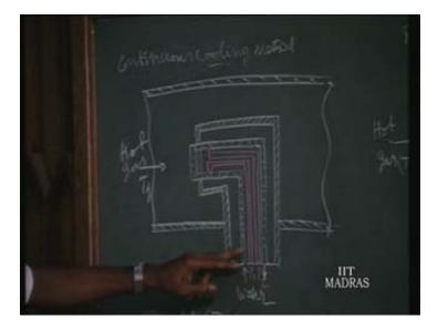
So measurement of higher temperatures higher than the melting point of one of the wires can be measured by adopting these two techniques, any one of these two techniques. That is called continuous cooling method; the other one is called pulse cooling method.
