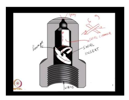
The next kind of design is again offshoot of this simplex nozzle and this particular design is, it simplifies a few different aspects of this simplex nozzle by making the passages fairly large. This is again a schematic, where the liquid is injected through the middle through this, what we are seeing here is sort of a cut section of the nozzle itself. And there is an insert this is typically called as swirl insert.
