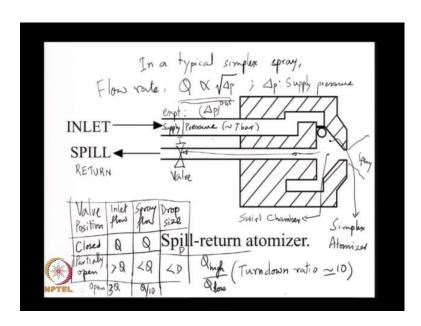
One of the features of all of these nozzles is that I have one fluid inlet that brings fluid into the nozzle and all the fluid that enters the nozzle is spread now as I increase the supply pressure.
