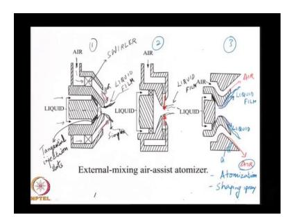
Up and till now, the source of energy remember we said that there are two things that this spray nozzle does; one it brings the liquid in contact with the source of energy that is essentially the objective of a spray nozzle.
