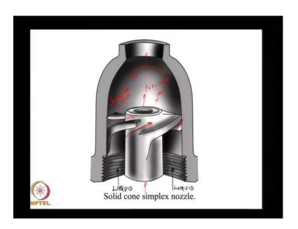
The liquid comes through this sort of an annular passage, and because of these vanes cause the liquid to be introduced into this region with a certain kind of a swirl action. So, you create a natural swirl inside this chamber that is going to be oriented in that direction; except you are also introducing some liquid directly through the middle through a center orifice of kind.
