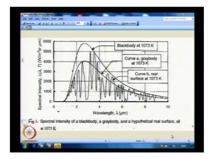
We are looking at this spectral intensity of a blackbody, gray body and hypothetical real surface all at about 800 degree centigrade, which is which is same as 1073 Kelvin. So, the top most curves is a blackbody at 1073. So, that follows the Planck's distribution. Then, there is a hypothetical surface which corresponds to curve A, which is a gray body.
