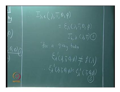
This equation can be used to experimentally determine epsilon lambda dash, if you want to do an experiment. That means, you have a complicated experiment, where you have a real surface, where you have a blackbody all that, so it can be used to determine epsilon lambda dash or more realistically or more practically, if somebody give an epsilon lambda dash equation 2. Let us you calculate I lambda e.
