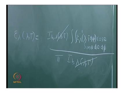
Now, substituting for e lambda in equation 4, we can do this. Shall I pull out the I b lambda, I can do that you have to do all this I. I will do that, what is the relationship between E b lambda and I b lambda (()) can I cancel I b lambda from the numerator and the denominator.
