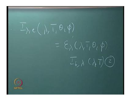
Now therefore, I lambda I am just re-writing. I will call it equation 2 for a given temperature wavelength and the given direction if somebody gives me epsilon lambda dash, either from theory or from experiments, I can use a Planck's distributions and get the I b lambda, multiply epsilon lambda dash by I b lambda and find out what is I lambda e.
