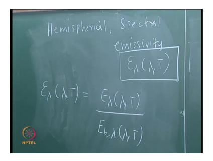
Now, first fellow is over now we will start integrating 1 by 1 hemispherical spectral emissivity. So, the hemispherical spectral emissivity is given by or we can do like this also is that spectral directional.
