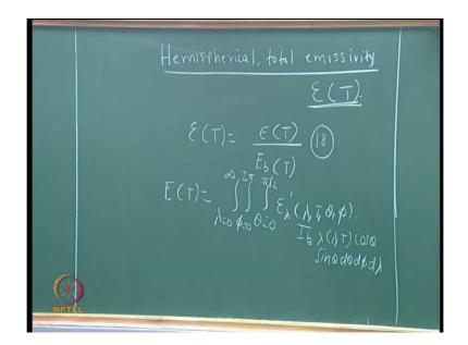
So, the lambda denotes that it is a spectral quantity, and dash denotes that it is a directional quantity. So, two directions are involved; the zenith angle and the azimuthally angle. So, namely theta and phi respectively; and lambda refers to be spectral, refers to the fact that it is spectral.
