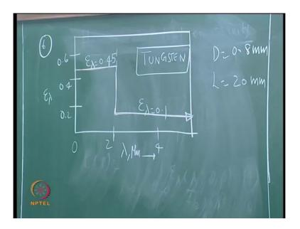
So, now let us solve some problem; problem number 6; and it is going on. So, arrow mark means it is continuously goes as 0.1 up to infinity; epsilon lambda, it does not stop with beyond two micrometer, it is having a uniform value or constant value of 0.1.
