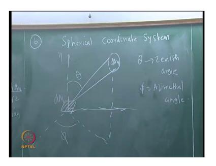
So, the first is solid angle. Next is we have to introduce a spherical coordinate system. So, what is a spherical coordinate system? So, let us consider, there is an elemental area d a one it is emitting radiation. It is going in all the directions. There is another elemental area d a n which is intercepting intercepting this radiation. So, this is the.
