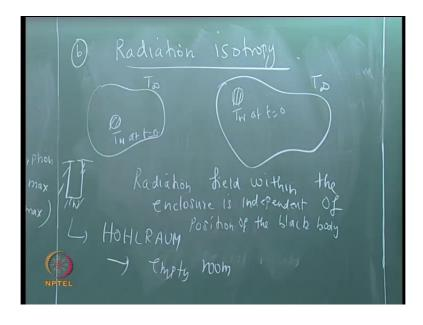
Radiation isotropy; if suppose the story is like this this T infinity T w or T equal to 0 right.
