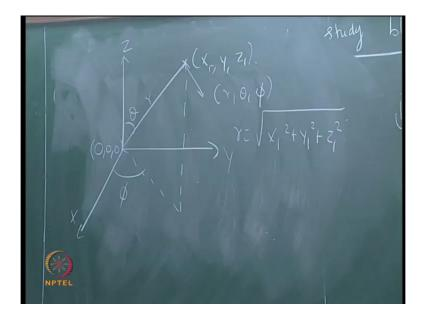
This you can on the coordinate system. You have now x y z some point which is given by x 1 y 1 z 1, this point can also be described the coordinates of this point as r theta pi, where r is basically of course, this is considered as 000.
