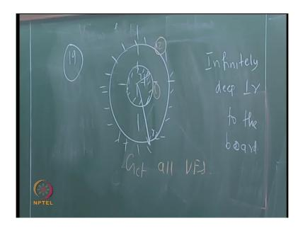
So, we will stop it at that stage. Now, do not worry about the radiation activity on the outside of surface two. Do not worry about the radiation activity on the inside of surface one. problem 19, was the cylindrical duct get all view factors. very good get all viewers, how
