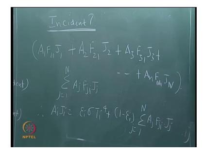
What is this incident coming from other surfaces; this is the question we have to answer. Sum of radiosities into view factors. Sum of radiosities into view factors, good enough, fair enough multiplied by the respective area, because I have put watts per meter square into. So, I will say incident could be, let us start with A 2. If, there is a self view factor it could be A 1 F 11 J 1 plus A 2 F 21 J 2 plus A 3 F 31 J 3 plus A n F n 1 J n. So, can we write it in a very compact form sigma.A j
