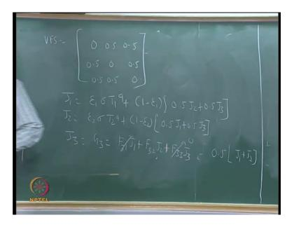
Now, because it is a equilateral triangle; F 1 1 plus F1 2 plus F 1 3 equal to 1, F 1 1 is 0, F 1 2 equal to F 13, therefore 2 F 1 2 equal to 1, F 1 2 is equal to half F 1 2 is equal to
