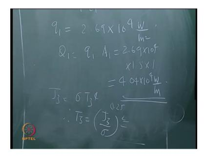
Now, q 1 is equal to, this is correct, we got the expressions for q in terms of G 1 as well as J 1, now you can write the expression for q 1. So, what do you get q 1, 2 point 69 into 10 to the power 4, Watts per meter square, this must be multiplied by 1 point 5 into 1, is 1 point 5 meters wide is it not? 4 point, 4 point 04.
