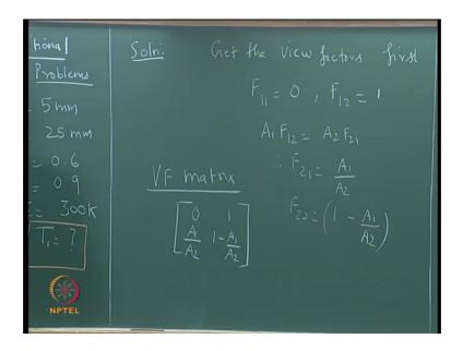
So, let us start, get the view factors first F 1 1 equals to 0, F 1 2 is equal to 1. So, first write out the view factor matrix 0 1. So, part A is over, first part is over. Now, we will write the radiosity relations.
