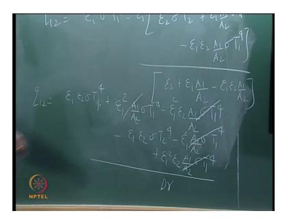
So, q 12, I erased the J 2. So, epsilon 1 epsilon 2. Sigma T 2 the power of 4. Plus epsilon 1 A 1 by A 2, sigma T 1 to the power 4 minus epsilon 1 epsilon 2 A 1 by A 2 sigma T 1 to the power 4, It is correct. Divided by Epsilon 2 plus epsilon 1 A 1 by A 2 minus epsilon 1 epsilon 2 A 1 by A 2 q 1 2 epsilon 1 epsilon 2 sigma T 1 to the power of 4, plus epsilon 1 epsilon 2 A 1 by A 2 sigma T 1 to the power of 4 minus epsilon 1 epsilon 2 A 1 by A 2, you are getting epsilon 1 square.
