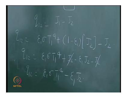
Substituting in equation 1. One would be J 1 minus J 2, so in equation 1 if you just subtract it on both sides. We can get the q straightaway, but that is what, we will write this, we can get or. Therefore, is that correct, that was good Vikram, otherwise you can find J 1 also, I cannot believe this, is this correct. I am now flying an autopilot I do not have this in my notes, let us see you should be able to see the runway.
