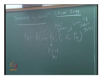
And, the Hottel charts – I have given to you for water vapors and carbon dioxide. These are... So, now, if you see epsilon g, that is, a gas emissivity should be a function of what all variables from your study of... of optical depth; instead of optical depth, can we start with mean beam length? Epsilon g – why should it vary on optical depth? Epsilon g need
