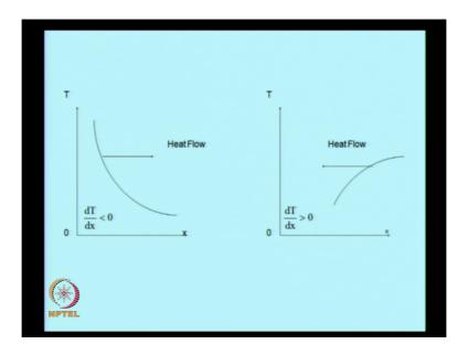
So, please note this very very important, if the temperature is decreasing along x and the heat is flowing from left to right, if the temperature profile is like this, heat is flowing from right to left, so you must get an idea of the direction. So, the direction is given by the second law of thermodynamics, which forbids flow of heat from a temperature, low temperature to high temperature without the application, without the aid of frictional work.
