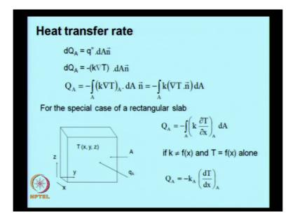
So, you can so you can say that the d Q A is basically this is watts watts per meter square, so the elemental heat transfer rate is equal to the flux into the elemental area. So, q can be replaced by k del T using the Fourier's law and then therefore, q must be integral d q over A, then you can do this k into del t into n, where n is unit vector.
