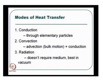
So, you we should not say this fag end of the course everybody knows that, there are three modes of heat transfer conduction through elementary particles, convection is advection plus bulk motion, but advection plus conduction, radiation does not require a medium it is best in vacuum. So, some people skip number 2 and say that that only 2 modes of heat transfer conduction and radiation, the elementary particles at high temperature regions at higher energy level oscillate.
