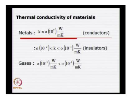
So, for metals the thermal conductivity is order 10 to the power of 2, for insulators its varies from 10 to the 10 to the minus 2 to 10 to the minus 1, gases it varies from 10 to the minus 3 to 10 to the minus 1, I will give you a table.
