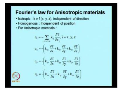
Now, there are some materials which are anisotropic, anisotropic material is one in which the thermal conductivity is independent of direction, that is thermal conductivity in x direction is the same as y is the same as z direction; if k x, k y, k z are found are dependent on the direction, it is called anisotropic material. A homogeneous material on one on the other hand, is the material in which the properties are independent of position.
