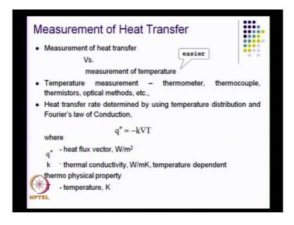
What about the measurement of heat transfer, why are we always talking about the measurement of temperature and not about measurement of heat flux, it is possible to construct heat flux gages, come up with the heat flux gages and so on. But, it is lot easier to it is a lot easier to measure temperature, because the various ways of measuring temperature you can use thermometer, thermocouple, thermostats optical methods, one of my student is working on liquid crystal thermograph.
