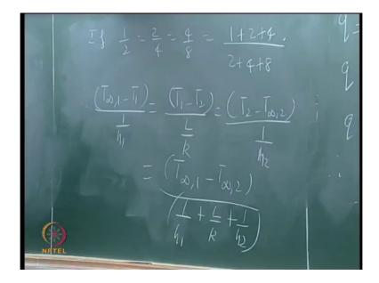
So, what it essentially means, is I have a temperature difference, global temperature difference T infinity 1 minus T infinity 2 between the two fluids. There are some resistances to the flow of the heat. The resistance is arise as the consequence of the finiteness of the heat transfer coefficient on the outside. The finiteness of the heat transfer coefficient on the inside. And the finiteness of the thermal conductivity of the solid.
