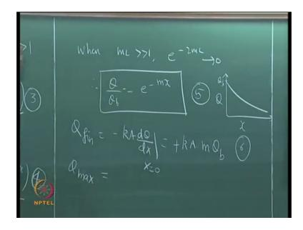
So, what is a Q max? The maximum heat transfer possible, the maximum heat transfer, which is possible from the fin occurs, happens in the whole fin, is at the base temperature. That is, t equal to t b throughout or theta equal to theta b throughout. Please remember, theta is a temperature excess t minus t infinity. So, this will this will be h PL to 7:40
