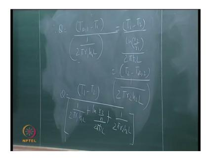
So, the 3 terms in the denominator are, the 1st term represents the convective resistance on the inside, the 2nd term represents the conduction resistance across the thickness of the tube and the 3rd term represents the convection resistance on the outside. The 1st and 3rd terms are also called as the, yeah, the 1st and 3rd terms are also called surface resistances. So, using the concept of electrical analogy...
