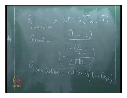
Now, what is a heat transfer rate? What is the L I am keeping, talking some L? L is the length in the direction perpendicular to the plane of the board. So, yes, ok.
