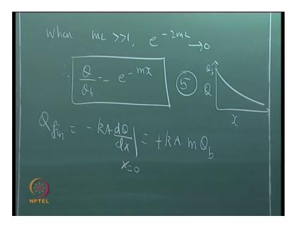
to 4:42 When ML, theta b by, theta by theta b e to the power of minus mx, it turns out to be a very simple case of exponential distribution. Even otherwise, the temperature distribution is exponential, but it has become very simple.
