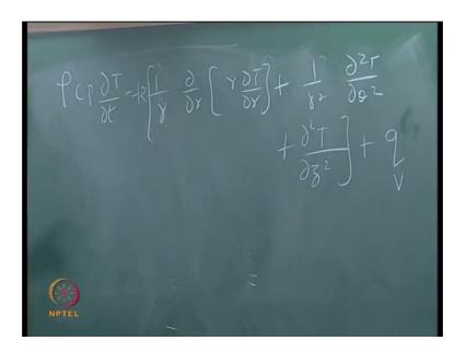
So, the governing equation for this will be rho Cp. to 26:42. This is for, uniform thermal, uniform thermal conductivity K. So, please note the essential differences between this equation and Cartesian coordinate equation; have you written this down? The essential differences are the left hand side is same as the right hand side, you got 1 by r dou by dou r of r dt by dr, we used to get d square t by dx square there.
