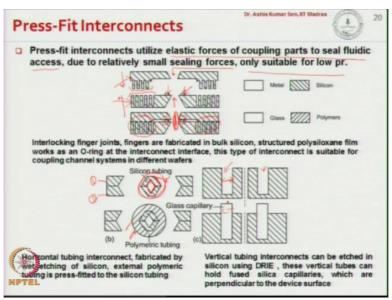
Now, depending on the interconnections the fluidic interconnections are categorized as press fit interconnection and glued interconnection. So, here will be looking at these 2 types of interconnection mechanisms. Now, first let us look at press fit interconnection, so the press fit interconnection basically utilizes elastic forces of coupling parts to seal fluidic access, okay and since it is based on elastic force, the sealing force is quite low.
