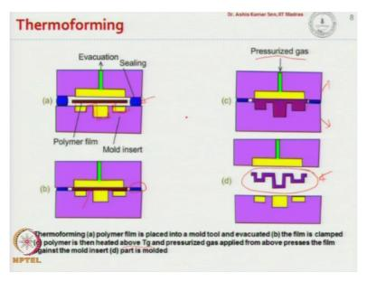
Then, we would have a multi-layer patterning on the surface and we can do it multiple time to create as many multiple layers that are possible, so that is known as micro transfer molding. Here, we talk about a process called thermo forming okay. In thermo forming; so this is the situation we have, here the polymer film is located inside the mold cavity, so this is the mold cavity.
