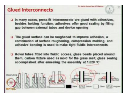
So and; because the polymeric coupler is you know, soft it can expand deform easily, we can get a better grip and fluidic sealing around the interface, so that is the reason we use polymeric coupler. So, this is so; you know this is a close of view of what happens typically in a polymeric coupler or sealing. Now, in some cases, you know the press fit interconnections or glued using adhesives.
