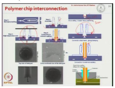
You can use things like glass beads and cure it at elevated temperature to create permanent and strong joints, so different options are available. So, here we talk about an interconnection system, so typically in; let us say in thermoplastic like COC microfluidic devices for fluidic interconnection, we normally go for nano port base interconnection, so in nano port based interconnection, we have this mechanism where we you know have a glue, which is solid.
