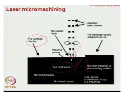
So, there are you know; various unwanted undesirable effects that come in, when the long pulse laser is used, so definitely long post laser are not suitable for fabricating micro channel structures. On the other hand, if we go for the ultra-fast laser pulses; in case of ultra-fast lasers, we do not have a specific melt zone here, so because the laser is very fast as soon as it falls, the metal in very locally gets evaporated and removed okay.
