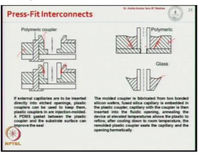
And typically, the diameter of these holes little bit smaller than the outer diameter of the capillary, so they can be pushed and fitted onto the hole. Here, we use you know; polymeric coupler for example, this is a polymeric coupler which is attached to the silicon substrate, so
