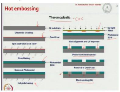
Now, we talk about the hot embossing process that we use for thermoplastics like cyclic olefin copolymer COC, so in this case we will talk about one example, where will be preparing a master, so for the hot embossing process, which is normally done once with say a cyclic olefin co polymer substrate, we will require a master okay which would have the configuration of the channel structure that we want to fabricate.
