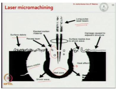
So, that is how, we can find for a given set of parameters, what is the minimum size of the feature that can be fabricated using lasers. So, here we see a typical you know; micro scan of a laser micromachining structure using long pulse lasers. So, long pulse laser as I was telling, it is not favourable but because it creates fex in the structures. So, when you have this long pulse laser comes in, it creates a melt zone.
