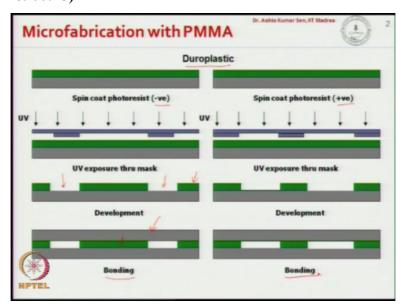
Okay, so let us continue our discussion on polymer based fabrication. Here, we talk about micro fabrication of micro channels with PMMA substrate; PMMA stands for poly methyl methacrylate, so it is a duroplastic as we have discussed earlier and so we start with spin coating photoresist on polymer PMMA wafer and so depending on the photoresist, whether it is positive or negative we end up with different structures.
