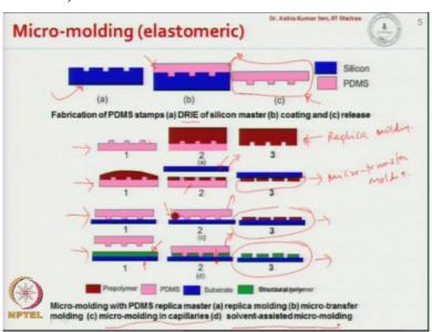
So, here we talk about micro molding using elastomeric substrate, so you know if you look at here, we take a silicon substrate that is; so this is basically silicon master which has a channel pattern, which can be fabricated using dry reactive ion etching okay, which gives straight channels and in the second step, we put a layer of PDMS on the tops which can be done using spin coating.
