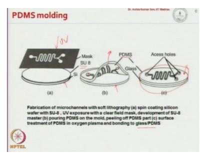
And when this master is taken out, we create a structure, a pattern on the surface of the substrate and this is known as solvent assisted micro molding okay. Here, we look at a typical PDMS molding based microfluidic device fabrication; it is starts with photolithography process, where you know SU 8 is patterned on top of the silicon wafer, so this is the Su 8; so this is the Su 8 that you see here which is pattern on the silicon substrate.
