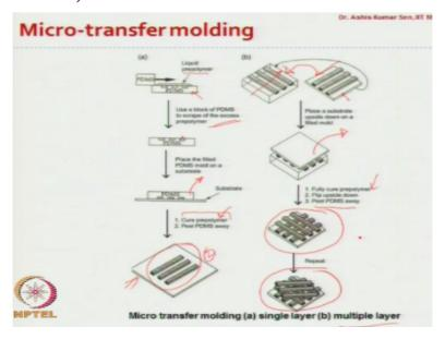
And then we can bond this PDMS open channel against a glass or a PDMS layer okay; a
