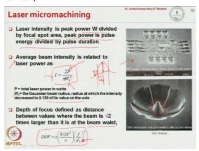
Because the pulse is very fast, so there are no surface debris as well because the metal get
