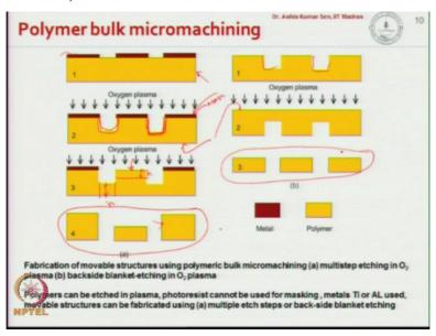
And then we remove this silicon layer away, so we have a double layer channel structure in this way, okay. So, here we want to create you know, movable structure using polymer bulk micromachining, so here we have the polymer substrate and which is coated with a layer of metal on top and then we go for oxygen plasma. The oxygen plasma basically removes this you know, the polymer where the metal act as a mask okay.
