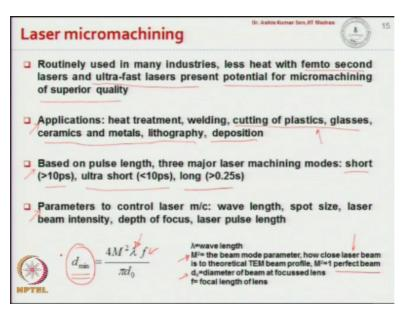
So, that is how the 3D part is going to be formed, so after the laser curing the parts are going to be cleaned by emerging in a chemical bath and then cured using UV, okay. So, that is when we get our structure. Next, we move on to laser micromachining; laser micromachining are routinely used in many industries and so you know, but one of the major limitations of lasers is that it produces heat.
