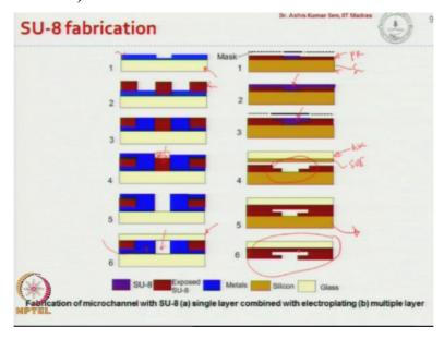
Here, we are using Su 8 photoresist as a structural layer, you know here we see the fabrication process, you know we have the glass substrate in this case, which is coated with some kind of metal okay and so this is the metal layer okay. So, you put photoresist here and then we metalize this further to fill out this cavity with metal and then we again metallized and pattern okay.
