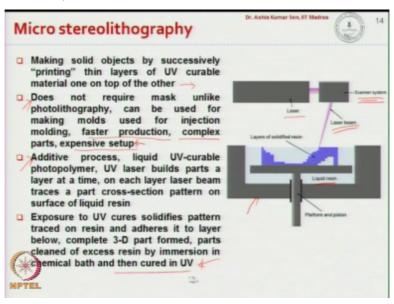
So, move on to next fabrication technique, which is micro stereolithography and in micro stereolithography, we make solid objects by successive printing thin layers of UV curable material on top of the other. So, this is what you have seen here; you see here, we have the liquid resin present inside this chamber and we have the laser; giving a laser beam and this laser beam is scanned onto this liquid resin layer by layer okay.
