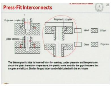
So, it will expand and get a very good grip around these areas, so we can achieve fluidic sale. So, here it again uses a press fit configuration using polymeric coupler and so you know here, we use a polymeric coupler and if you use pressure, so if you use pressure the polymeric coupler will expand and fill this gap here okay. So, this gap is completely filled here and now we choose a capillary whose outer diameter is more than the inner diameter of the polymeric coupler.
