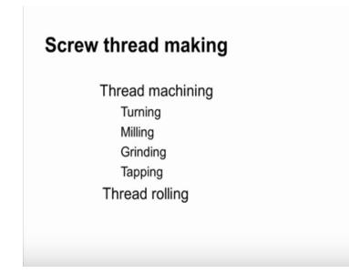
Now, how these threads are made there are many methods. The very common method is the thread machining they can be turned, they can be milled and thread grinding thread, tapping, so these are some trade machining methods and the threads can also be made by a thread rolling operation.
