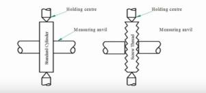
Now I can see here, S is the diameter of the standard cylinder normally plain plug gauges are used as standard cylinder and R1 is the reading on the standard cylinder and R2 is reading on the thread to be inspected and then D the major diameter of thread can be calculated using this relationship S+ or -R1-R2. Whether we use + or - it depends on whether the standard the cylinder diameter is > the major diameter of thread or < the major diameter of thread.
