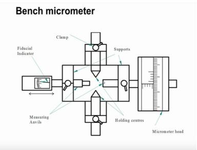
So to apply even pressure for all the work pieces this fiducial indicator is provided and on this table surface we can put some fixture to hold the work pieces. Now this shows a schematic diagram of for bench micrometer. The micrometer head with the scale on the thimble and we will scale on the barrel and then we have the measuring anvils and clamps for measuring anvils fiducial indicator the anvil and fiducial indicator it is slide.
