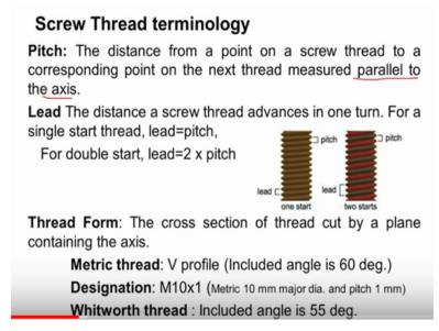
Now pitch it is a distance from a point on a screw thread to a corresponding point on the next thread measured parallel to the axis this is very important when they measure the pitch measurement should be made parallel to the axis. Now you can see here this is a single start screw thread so we are in the lead = pitch.
