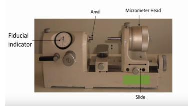
Now let us the study how the major diameter of a screw thread is measured this instrument is known as bencher micrometer, we can see the very rugged caster and the base of the instrument wherein there is a slide which can be moved or parallel to the axis of the bench micrometer this is slide the body which houses the micrometer head a large diameter micrometer is fitted and is a anvil so when they rotate this symbol the anvil moves in or out.
