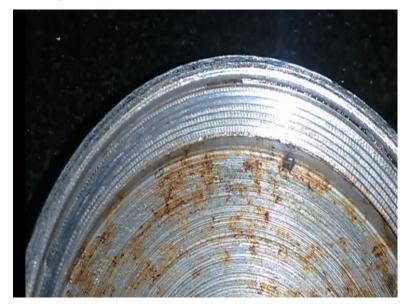
We can see a component having internal threads you can see here these are the internal thread now we are required to measure the minor diameter of a internal thread. So for this I am using 2 steel balls and slip gauge box, initially we should measure the approximate minor diameter using a vernier caliper.
