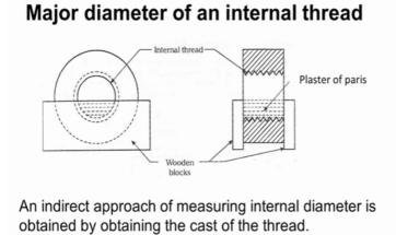
Now measurement of major diameter of internal thread, so for this we use a method called casting method you can see in this diagram this is a work piece having internal threads, whose measure diameter is to be measured. Now we have to take a replica of for this internal thread, so how do we get the replica of internal thread, you can see rearrangement.
