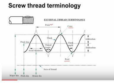
Now let us move to the screw thread terminology various terms are used in the respective screw threads internal screw threads and external screw threads Now this picture shows some of the terminologies you can see the profile of the screw thread and the distance between one point on the screw thread to the corresponding point on the next thread this is the known as pitch.
