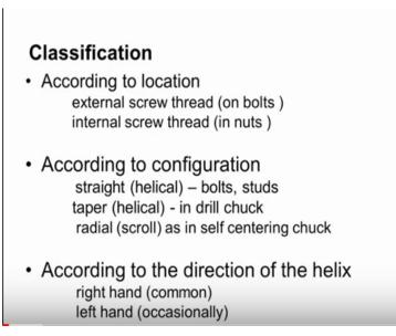
Now, let us study how these the screw threads are classified they are classified according to the location that means that is whether these screw threads are made on the external surface as in bolts or whether they are made on the internal surface of example nuts. These threads are can also be classified according to the configuration.
