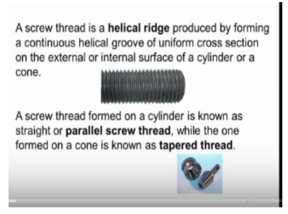
It is basically a helical Ridge produced by forming a continuous helical group of uniform cross section on an external or internal surface of a cylinder or a cone. Now, you can inspect for photo we can see the helical ridge produced and a cross section use the uniform for all the threads now
