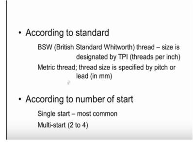
According to the standard BSW British standard Whitworth thread or metric thread according to the number of start ordered a single start or double start like a multi start screw threads.
