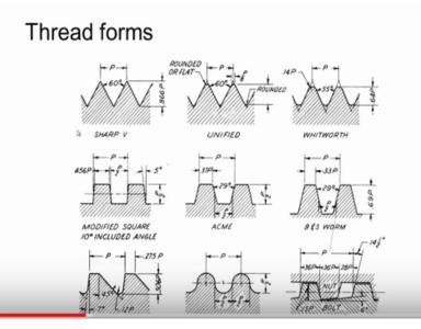
Now various thread the forms are used in the practice is sharp v, we have a sharp crust here, so it is a slightly modified it is made rounded or flat then it is called unified thread and then the in 2 cases a sharp and in unified the included angle is 60 degree, whereas in the case of whit worth thread the included angle is 55 degree and then modify the square 10 degree included angle these are modified square threads used in power screws.
