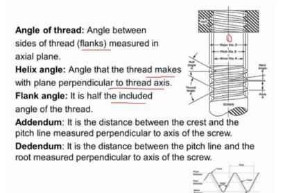
Now angle of thread so angle it is the angle between sides of thread that means angle between 2 flanks measured in axial the plane you can see here we have a flank, flank here. We have another flank here so the included angle between 2 flanks is known as thread angle and helix angle is the angle that the thread makes when with planes perpendicular to the thread axis. So this is the thread axis so we have the thread axis here and then this is the ridge or the thread okay.
