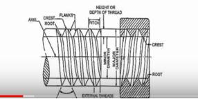
Acme matrix wherein the included angle is 29 degrees, similarly we have modified buttress and the knuckle threads so like this different threads forms are available. Now what is the major diameter, we can understand from this diagram the it is the measure diameter is the diameter of an imaginary cylinder co-axial with the screw which just touches the crests of an external thread you can see here we have the crest points here.
