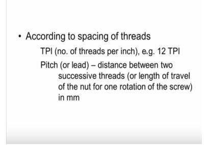
According to the standard BSW British standard Whitworth thread or metric thread according to the number of start ordered a single start or double start like a multi start screw threads. According to the spacing of threads I can say TPI thread number of threads per inch, whether it is 60 TPI or 12 TPL like that we can classify and depending upon the pitch also.
