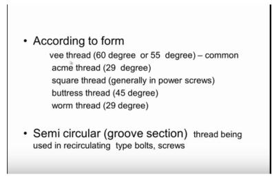
According to the form they are classified as the vee threads normally 60 degree and 55 degree thread angle is used acme thread wherein the angle is 29 degree they are classified as square
