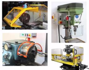
Now is the machine adequately guarded? Guarding of the machine also we should check. We can see the different kinds of guarding are used in the machine tools the guard provided for lathe and other type of guard transparent guard provided on the lathe this is the guard provided for the pillar type drilling machine and the guards for milling machine.
