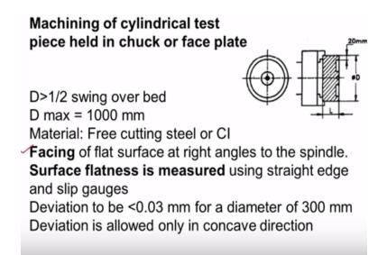
Just now in the 2nd test facing operation is performed. Here the work pieces mounted in a chuck or faceplate. That the diameter of the work piece is should be greater than half of swing over bed. If swing over bed is 100 millimeter then the diameter of the work piece should be greater than 50 millimeter and D max should be 1000 millimeter if swing over bed is more than this particular size and then the material work piece material free cutting steel or cast iron.
