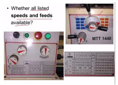
Then we should see whether all the listed speeds and feeds are available. we can see many spindle speed like 1170 rpm, 385 rpm and lowest speed such as 165 rpm, 90 rpm they are mentioned in the display we should do the settings of the gear and we should use in an appropriate speed testing device to check.
