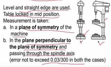
Now we are going to conduct the flatness of the table surface also the flatness of the base plate of the machine. Bass plate of the machine of the mission the surface is also t slots and it should be pillar and we have to check whether this base the machine base is flat or not for measuring the flatness we can use the precision level or which is shown here or we can you straight edge and gauge blocks along with the feeler gauges these instruments can be used to check the flatness.
