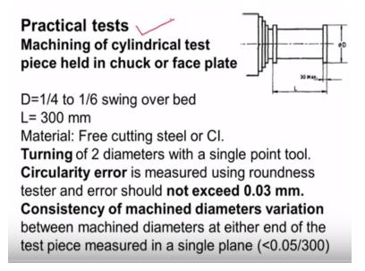
Now we will discuss about the practical test conducted on engine lathe in which the work piece is mounted in a chuck or faceplate. Mounted on the mouth of the late spindle and machine comprises in which phasing and turning are performed and the machine accuracy is tested. In this diagram you can see work piece of length 300 mm mounted in a chuck or faceplate the diameter of the work piece is 1/4 to 1/6 of swing over bed.
