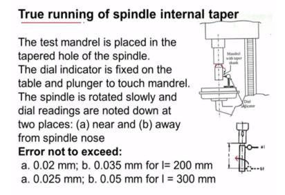
Text, now other important test that is conducted is true running of spindle internal taper here we have the spindle of the drilling machine this is the spindle and inside there will be tapered board this is the axis of the spindle. Now the spindle internal board or internal taper should run through this .insert the drill bit in the taper so if this internal taper is not true then the drill tool will wobble it will verbal and we do not get a proper drill hole.
