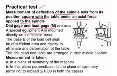
Now let us discuss about the practical test that can be conducted on this type of drilling machine. Actually it is measured the deflection of the spindle axis from its position via with the table under an axial force applied to the spindle or for conducting this experiment we use dial gauge and broad gauge.
