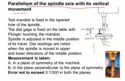
Now we will discuss about the parallelism of spindle axis with its vertical movement spindle we move up and down for feeding the drill tool into the work piece the movement vertical movement of the spindle should be parallel to its axis. If the access this is the spindle axis and the spindle movement is at some inclination then what happens is when we see the tool we get a hole at some inclination of we do not get the drill hole.
