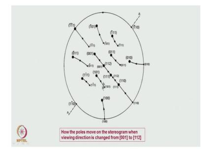
This is what is shown as an example, like what I mentioned that you have to. See this is for the case of 112 the pole is being brought to the center, this about 36 degree when this is being rotated, in the same direction on this equatorial plane 001 is rotate then it reaches here all others because the rotation axis now is around this 11 bar 0 in this axis then if we rotate around this axis this is going to be the equatorial plane.
