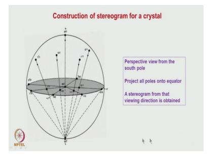
That is what is being shown in this stereogram, in this view graph. Here you can see that these are all the various poles. And all this poles also should as we have discussed in the last class the angular relationship between the various poles which are lying on the surface of the sphere that is being maintained here. And if you see this projection plane that is; what is the stereographic projection; that is the projection plane which is shown here.
