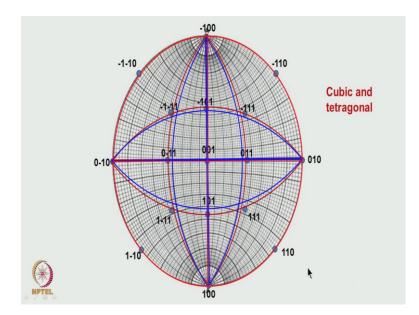
So, once we have a table like this like we constructed the stereogram using this information we can construct a stereogram for this tetragonal crystal also. That is what is essentially shown here, here what is going to happen between 001 and 100 it makes an angle which is essentially of around 39, there is from 001 and 101 its 39. So, since it is lying on a longitude we can directly mark it, between 100 and 101 its 50, so this is the point which it will come.
