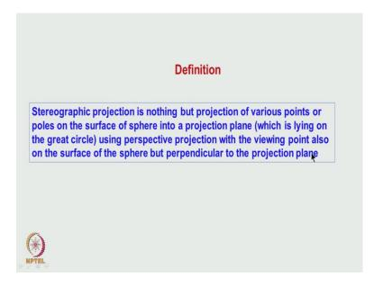
What is the basic definition of stereogram? I mention first the beginning the stereogram is nothing but a perspective projection, but its conditional one. The stereographic projection is nothing but projection of various points on poles on the surface of the sphere into a projection plane and the projection plane is lying on a great circle and using perspective projection but the viewing point also on the surface of the sphere, but perpendicular to the projection plane that is what essentially.
