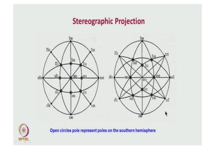
In this particular projection what I am showing it essentially is the 001 projection is being shown. And here if you see the two circle which you can see the once which are field circles they are corresponding to the poles which are lying on the top hemisphere. If you wanted to project the poles which are lying on the bottom hemisphere then what we have to do it is that all those poles will be marked with a open circle. That is what essentially it is being shown here.
