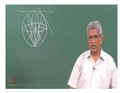
This is nothing but if this is sphere, if this is one of the projection plane then if we are giving from this direction all the points on this hemisphere they are projection they cut this equatorial plane this points are the once which show the angular relationship in three dimensions which is nothing but the angular relation three dimension which is projected on to a two dimension.
