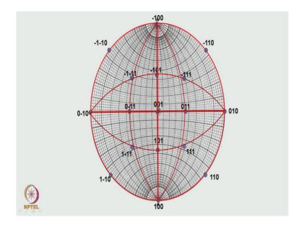
What has essentially been done is that since we are drawing stereogram is 001 the 001 will come at the centre of the stereographic projection. So, what we have done is taken the Wulff net on top of it we have kept a stereogram, drawn the primitive circle, and then mark this two axis x and y, mark this point at 001. By convention 100 direction as to come here down and the 010 direction has to come in that y direction.
