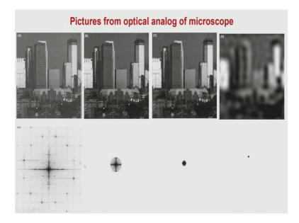
This is an optical analog picture which has been taken you see here we have the skyline of a photograph which is there; which is taken analog film in an optical analog; what is being done is that instead of an electron beam which we use it in a microscope what should be the characteristics of the beam you should be monochromatic and coherent the same type of beam in optical radiation we can achieve it using lasers.
