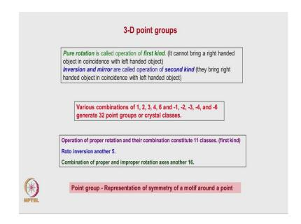
So, essentially how many symmetry elements that is rotation if you consider there are 5 mirror 6 right, then roto-inversion these are all the symmetry elements, then I combination of roto-inversion and rotation axis, all of them put together if we see the total number as I mentioned is 32. What I will just describe briefly is so far we looked at only just the stereographic projection of it.
