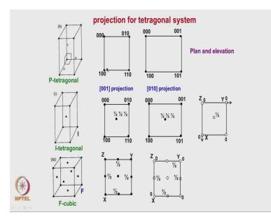
So, you look at the crystal then try to represent it in 2 directions you look at it. So, this is a projection which is given now of the crystal looking along 0 0 1 direction this is how it looks correct for a tetragonal lattice and this is how the projection which it will be in 0 1 0 direction correct. Once these 2 projections are given the crystal is completely specified the lattice is come where the unit cell of the lattice is completely specified correct complete information is available.
