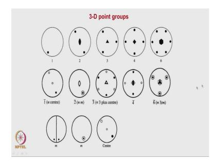
So, that is what essentially I had shown it here, this is a an 1 fold symmetry, then a 2 fold symmetry that a point which we take that is rotated once 180 degree and then again rotated this is a symbol which corresponds to 2 fold symmetry; like this we can have 3 fold, 4 fold, 6 fold. So, far we have considered the various symmetry operations like rotation, mirror, inversion, screw and glide all these operations can be represented.
