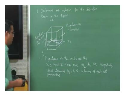
So, let us go to this problems for todays tutorial. So, what I have drawn here is, this is a cubic unit cell and then you have the sides a b and c. And the question is determine the indices for the directions shown in the figure, the this is the direction we are going to determine through the set of procedures you have already seen in the lecture.
