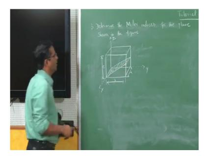
So, determine the miller indices of the plane shown in the figure. So, this is the plane let me shade it. So, I have put a b c need not be a cubic crystal could be a orthorhombic crystal or any excel which is having a different dimensions parameters altogether, but a plane of this kind how do you find the or how do you assign the miller indices. So, you must have gone through the procedures in in the lecture notes.
