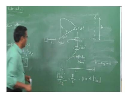
So, what you are seeing here is the geometrical nature of the di fraction pattern. So, you can write this relation g h k l by 1 by lambda is equal to r by l or we can write r is equal to. So, you can use this simple relations to solve some of the problems which we have given in the assignments. So, I would like you to post the questions if you have any doubt then we will take it up in the next tutorial class.
