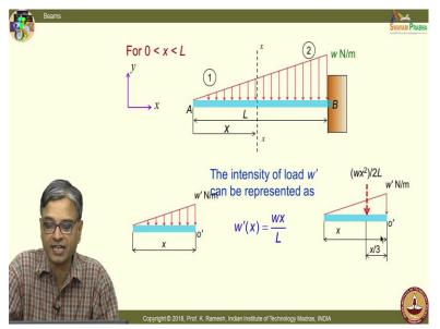
how to find out the centroid as well as the area, one can easily find out the resultant and that acts at the centroid which is at a distance x/3 from the base.
