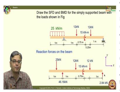
of bending moment diagram, the interrelationship is dM/dx = V and V is negative. So, I expect the slope to be negative. So, that gives a verification that we are on the right track and to plot the curve whether this way or the other way. It is better that you find out what happens at the centre
