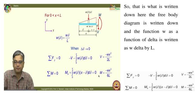
So, that is what is written down here the free body diagram is written down and the function w as a function of delta is written as w delta by L.
