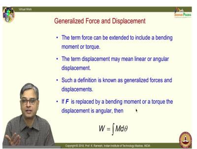
And I have this as *ds*, when I put this as simple *d*; we are talking about real work not virtual work. So, when I move this the force has moved, but the force and the displacement are mutually perpendicular to each other. So, it does not contribute to work you can also look at as a reaction force you can also look at
