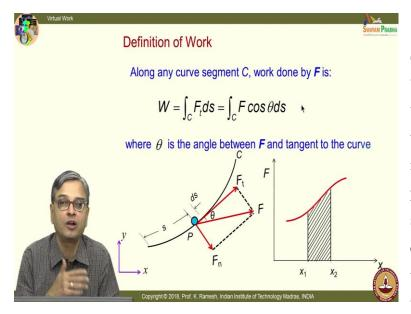
Suppose I want to know what is the work done when it has moved along the curve? I simply do the integration of this over the path and this also you have studied earlier. And you can find out work done as the area under the curve, when you go from one
