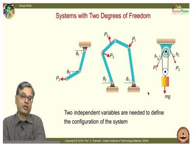
introduce one more linkage, the four-bar linkage was like this it is enough that I specify theta the configuration of the system is completely defined.
