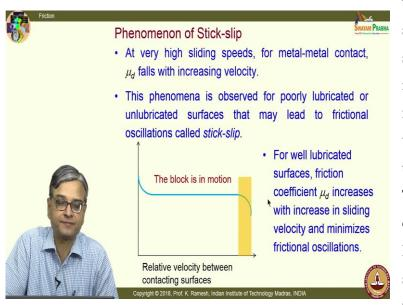
the symbol  $\mu$  with the suffix d. At very high sliding speeds for metal to metal contact  $\mu_d$  falls with increasing velocity this is what is observed. What is the consequence of it? These phenomena are observed for poorly lubricated or unlubricated surfaces that may lead to fictional oscillations called
