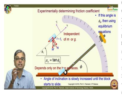
that position and you have to employ that for applying your frictional laws. When I say frictional force is proportional to  $\mu N$ , it happens only when the motion is impending that is very important to see. The first case I have Perspex on Perspex, the frictional it is very smooth I have a smaller angle that is about
