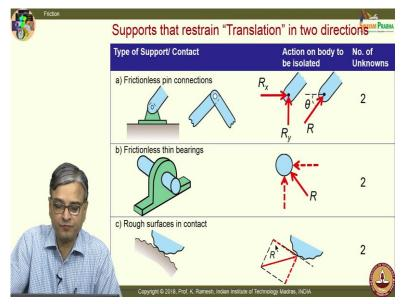
you have two reactions the force is unknown and the direction is unknown. So, you have essentially two unknowns. We also saw frictionless thin bearings, here again the direction as well as the magnitude are not known you have two unknowns.
