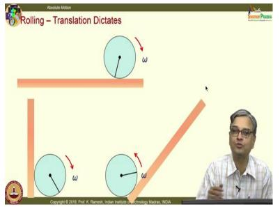
have to accommodate rolling from the fundamental principle. You have to recognize rolling is a combination of fixed axis rotation plus a translation; it has a rotation and a translation.
