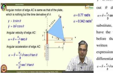
$\dot{y} = b\dot{\theta}\cos\theta$ , so I can find out  $\theta$  dot. So, I get  $\omega = \dot{\theta} = \frac{v_A}{b} \sec \theta$ . So, when I substitute, I get this as I have the values also, but before that I have also down the expression alpha; for differentiate this again  $\alpha = \ddot{\theta} = \frac{V_A}{b}\dot{\theta}\sec\theta\tan\theta$ And
