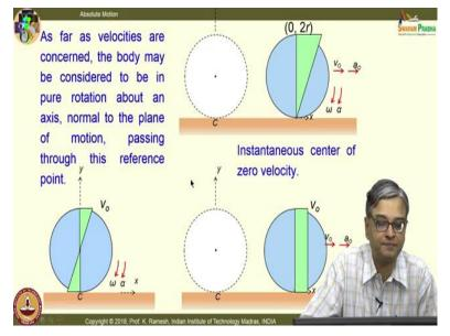
What is the meaning of it? It is as if the object rotates about this point at that point in time; I have a variation of velocity like this; this is very similar to what I have done it from the centre to this, from the center to this I have put a triangular variation; this was the axis about which it
