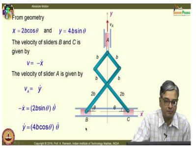
it is going to when I move up C will be in the negative direction; C will move in the negative direction the axis of  $-\dot{x}$  and we have a  $X = 2b\cos\theta$ relationship So, the velocity of slider A is given by  $-\dot{x} = (2b\sin\theta) \theta$ and  $V_{\rm A}$  is y  $\dot{y} = (4b\cos\theta) \dot{\theta}$ dot and
