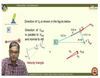
in the previous sketch is in this direction. This perpendicular this to connecting rod I have velocity of G with respect to B. When I close the vector polygon, I get the velocity of G and that is what is shown there in the actual point, we can also determine the magnitude now.
