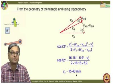
For that I again I need to do properties of the whole diagram. So, I need to find we already know the angle 72°. And I can write from knowledge of trigonometry cos 72° as a function like this, so, you have to go back and brush up your basic trigonometry properties of triangles
