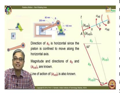
have already told you, because its reciprocating like this. So, I can put this as a horizontal line and we know we absolute acceleration of point B. So,  $a_B$  is known and the relative acceleration of the normal component is also known, normal component is known like this and your tangential component
