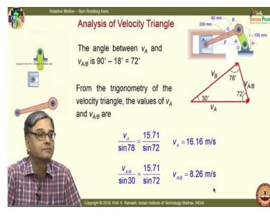
respect to B are determined as follows. I have  $\frac{v_{A}}{\sin 78} = \frac{15.71}{\sin 72} \quad v_{A} = 16.16 \text{ m/s}$
