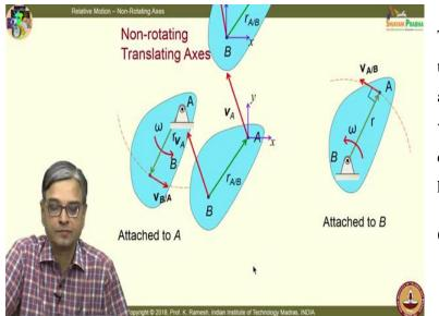
The idea of attaching a translating axis at B amount to translating with velocity  $V_{\rm B}$  and you have a corresponding rotation here.
