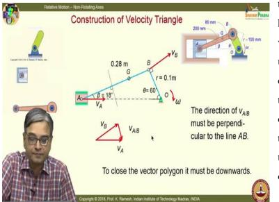
So, I know how to put the direction of the relative velocity of A with respect to B, this is
