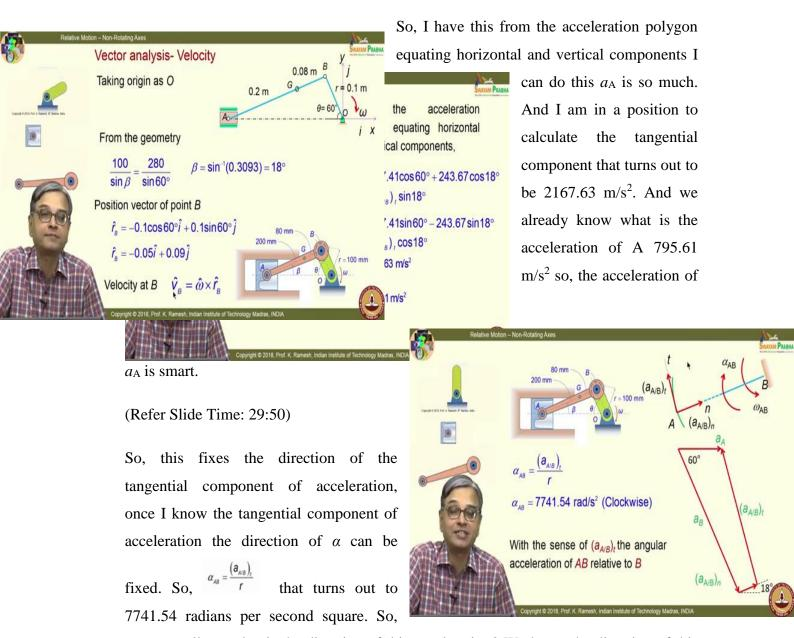
can you tell me what is the direction of this acceleration? We know the direction of this with the sense of  $a_{AB}$  that angular acceleration of a *B* relative to *B* can be determine.
