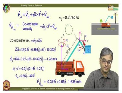
but rewrite this expression specific to the problem of interest because A and B positions are interchanged. So, I would now rewrite this as I have to get velocity of *B* with respect capital XYZ. to And this replace term as coordinate velocity. There better is a way of understanding it. So, I am
