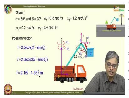
instances you again invoke only circular motion equations in different forms. Circular motion equations are very useful. Here, again because this is rotating like this. I will again use that kind of expression for me to find out, what is the velocity of **B**?
