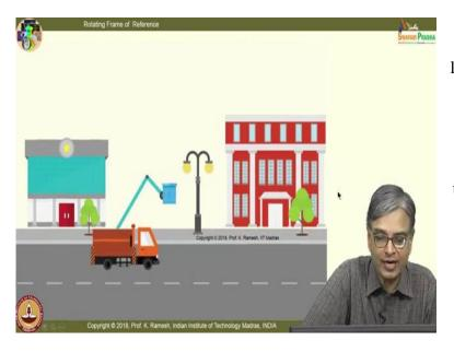
have a norm here, I have labeled this as A, I have labeled this as B and I have a platform attached at *C*. And the platform is such itself aligning, whenever the arm is having a motion like this it will self-align itself. So, that the person standing here will remain horizontal and he is in a position to do the job.
