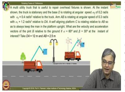
acceleration angular  $\omega_2$ dot. And here this arm is pinned here and this is rotating with angular velocity  $\omega_1$ . This also have an angular acceleration  $\omega_1$ dot and here, I have deliberately modified the symbol. So, that you also get to know, how to write the expression? You are
