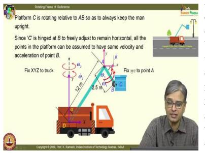
And where do I fit them? So, you are given this alpha is at 60° and  $\beta = 30°$ . You are asked to find out the velocity and acceleration vectors of point B. It is put as pint, its point *B* related to the ground and you are given this length of the member as *DA* equal 12 meters and
