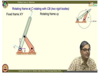
position to remember that. And it is fairly easy to solve this and I get this  $\hat{a}_{rel} = -14614.2^{\circ} \text{ mm/s}^2$ . We have used a very important understanding, that the  $a_{rel}$ would be along the slot. It is dictated by the slot. It is dictated by the slot. I will put it that way because if the slot is curved then it can have a normal
