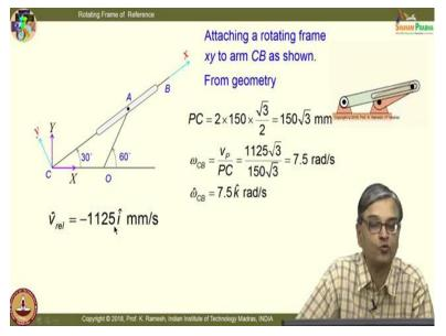
So, if I have x is positive this way, when it is coming  $\hat{v}_{rel} = -1125\hat{i} \text{ mm/s}$ down And from geometry, we have already said that point P and A are coincident. So, I can find out PC $PC = 2 \times 150 \times \frac{\sqrt{3}}{2} = 150\sqrt{3} \text{ mm}$ And we have already got what is  $V_{\rm P}$ . We know the length
