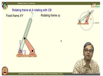
direction of velocity as well as the acceleration direction. Slot, if it is straight, it turns out to be along the slot. If it is curved, it is dictated by the normal and tangential components.
