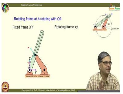
have two members are rotating. I have a crank *OA* rotating and also the slotted member *CB* is oscillating.
