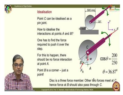
this plane. So how can I idealize the joint here? I can idealize the joint as a pin joint, but before I do that, I should also label my key points on the diagram so that it is easy for us to document whatever that we want to do.
