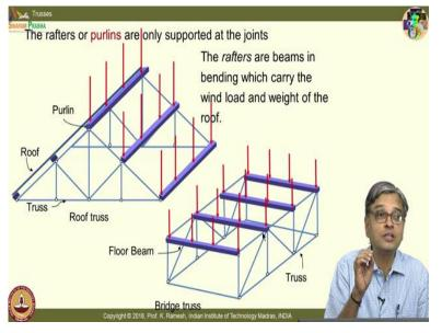
So, if I have to idealize this as a truss, I should apply loads only at the joints; that is cleverly done by a combination of beams and trusses. Here you have a road and you call that as a floor beam, and floor beam is having a transverse load. And this floor beams are supported at the joints of
