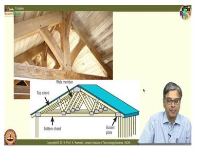
The members forming the truss are subjected to axial loads; that is very important to notice, though the external loading is in the transverse direction. I have the truss; I have the loads which are transverse to the truss. But if you look at the members; the members be may in
