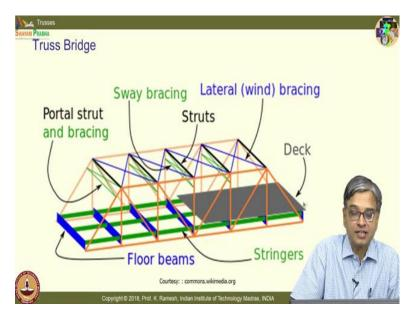
And you know we had seen in our introductory lecture, failure of Tacoma's narrow bridge. And I said that was because they have not taken into account the effect of wind forces while designing the bridge. And you could see here a typical design of a bridge truss with lateral bracing
