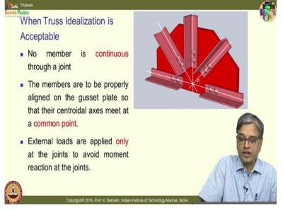
I have this as a roof truss and what I have is I have these rafters and these rafters are cleverly supported only at the joints. They are also called purlins, and they take the wind load and the load due to snow. So, these rafters bend whatever is the
