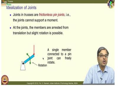
single member connected to a pin joint can freely rotate; it cannot support a load. However, when I have an array of members connected by pin joint, we would see what happens to them, how the members are connected is very important. So, what you recognise is, when you
