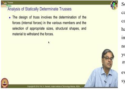
So, m+r=2j is satisfied, can this truss be stable? It cannot be stable. Unless I have the members arranged in this way; the truss will not be stay stable. So, what you will have to look at m+r=2j is satisfied for every conceivable subsystem.
