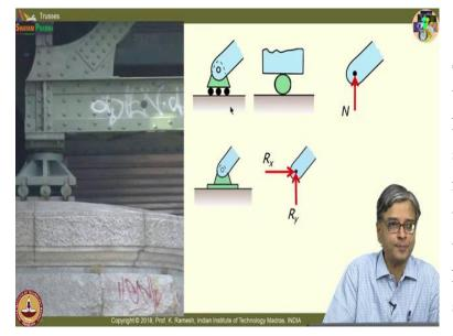
So, we have seen in one of the classes earlier, how a huge truss bridge is supported on rollers. And from analysis point of view we need to know what are the unknowns that we have how do we model these supports. We have already seen; the roller support can
