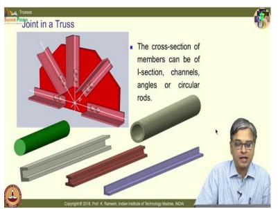
If you go and supervise any of those structures you must ensure if you want to make a truss the members should be aligned properly and another aspect you should notice no member is continuous through a joint. If a member is continuous; then it behaves like a beam, we do not want the members to behave like a
