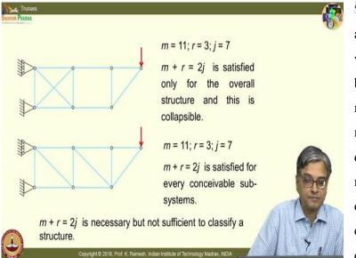
m + r < 2j and you have already seen how the truss was behaving. It was like behaving a mechanism; do we need mechanism? Yes, Ι definitely need mechanism. If I have to draw parallel lines in my drawing, I need a mini drafter; mechanism is also
