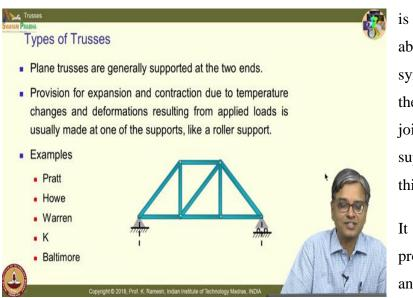
have a support like this, it is a symbol; you should be able to interpret this symbol correctly; what is the symbol? This is a pin joint. And how is it supported on the other end; this is on a roller support.
