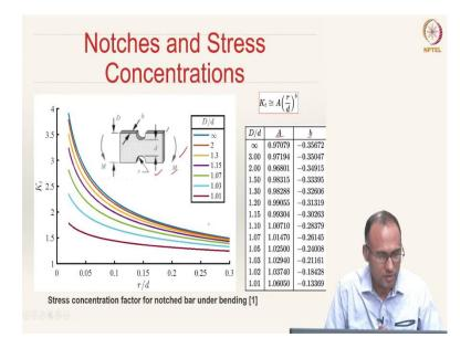
Similarly, if you are applying a bending moment, not on a circular cross section, but a rectangular cross section with these geometry dimensions, again you need to come up with new values of A and b and then, depending upon the load you have these concentration factors.
