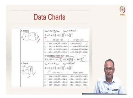
The material is subjected to both bending and twisting, but we know that the stress concentration factor changes depending on the type of load that is being applied and hence, you need to look for stress concentration factor due to bending separately, due to twisting separately.
