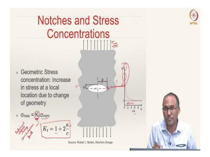
Let us take one example. If you have an infinite body -- so, here this shape actually means that the body is pretty long and you have applied a far-field stress, far away from an elliptic hole. This elliptic hole is described by semi-major axis a and semi-minor axis c. Then, the maximum stress near the notch i.e., the elliptic hole boundary is given as,
