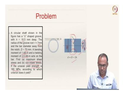
Let us solve one problem. Here you have a circular shaft of diameter d and then, the "U" shaped groove with h = 10.5 mm; that means, the groove diameter is 10.5 mm deep. The radius of the groove is 7 mm and the actual diameter is D = 70 mm. On this shaft, there is a bending moment as well as twisting moment; there are two loads that are there.
