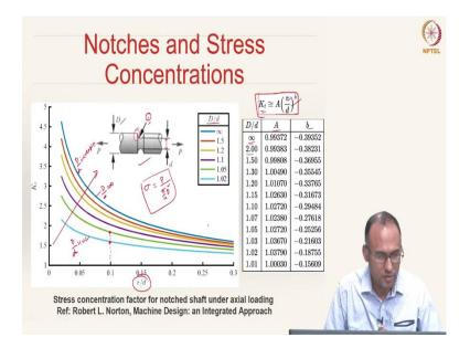
The stress concentration factor depends on the geometry and the loading. Consider a shaft subjected to an axial load with a diameter D with a groove radius r. If the applied load is P, then the nominal stress,
