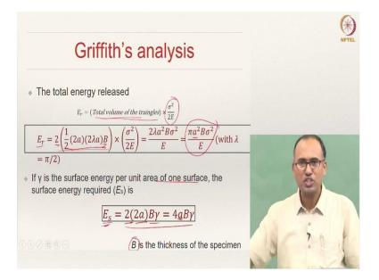
Since we are only considering linear elastic materials, the strain energy density i.e. the strain energy per unit volume of the material is  $\frac{\sigma^2}{2E}$ . We have done that in the previous modules. Let us assume that *B* is the out-of-plane thickness.
