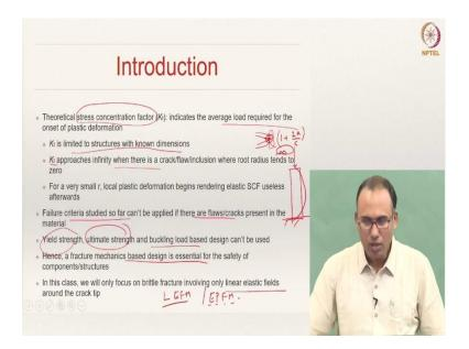
In the last class, we have talked about something called stress concentration factor, right? When you have a crack like defect, a hole -- we have seen the example of an elliptic hole, we have also seen the example of a notched bar. There we have defined something called stress concentration factor.
