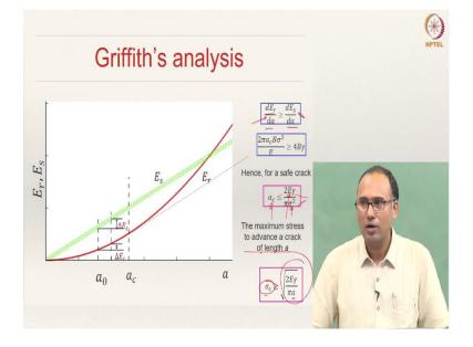
The released energy scales as  $a^2$ ; that means, it is a parabola and surface energy is proportional to *a*; that means, it is a straight line. What Griffith said was, when the energy release rate becomes greater than the surface energy rate -- here when we say rate, it is not time rate, but it is energy released per unit crack length.
