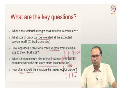
What are the key questions to ask having understood how a crack behaves? We said as you increase the length of the crack, the residual strength of the component reduces. What is the residual strength as a function of crack size? Can you actually relate these two things? The second question to ask is what size of a crack can be tolerated at the expected service load.
