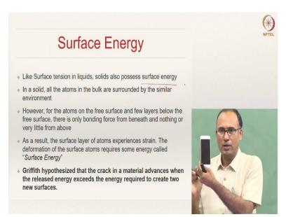
What is happening when you are cutting a slit to the system? You probably heard of surface energy, right? Like surface tension for liquids, for solids we have something called surface energy. It is reasonably easy to understand.
