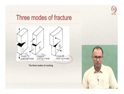
When we are studying fracture, you have three modes of fracture: mode I, mode II, mode III. Mode I is also called opening mode. Let us say this is the crack face and the load is applied perpendicular to the crack face. Because the load tends to open the crack surfaces, it is called opening mode. Mode II is called shearing mode or sliding mode. The load is parallel to the surface you can see. Mode III is the tearing mode.
